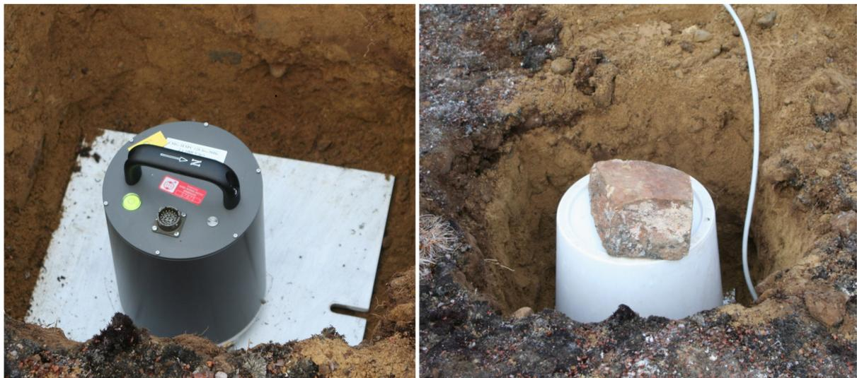
Fig. 9.12: Set up of the seismometer of land station 450stL2 on a wooden plate (left) and plastic bucket with stone to shield it from temperature changes and wind (right)
