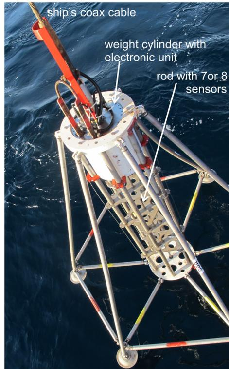
Fig. 10.1: BGR - hard ground heat flow probe
