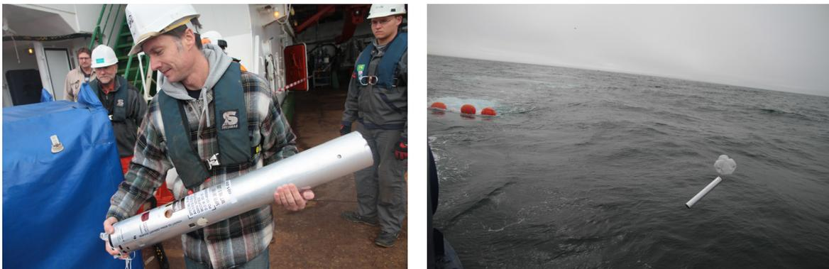
*Fig 9.8: A sonobuoy before and directly after deployment from the ship*
