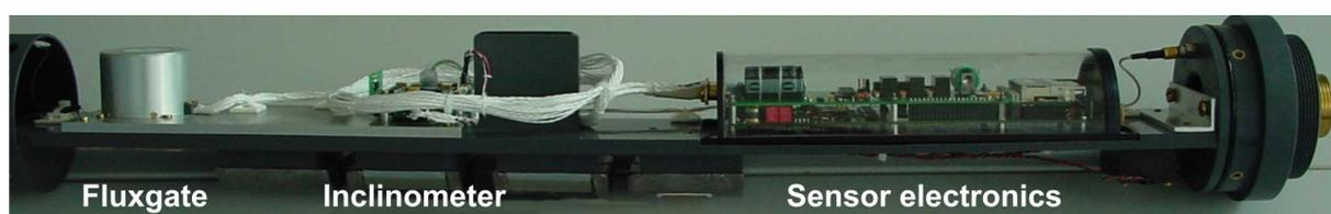
Fig. 8.2: Components inside the fluxgate magnetometer tow fish.
