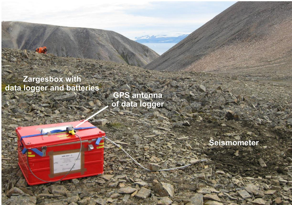
Fig. 9.11: Set up of land station 300stL2 equipped with a broadband seismometer
