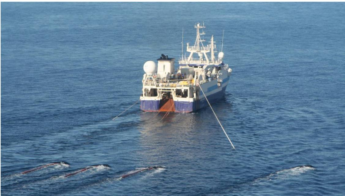
*Fig. 3.1: The seismic exploration vessel M/V Bergen Surveyor in the Melville Bay - Seismic operations of this vessel and Polarstern had to be coordinated to prevent interferences in seismic data.*
