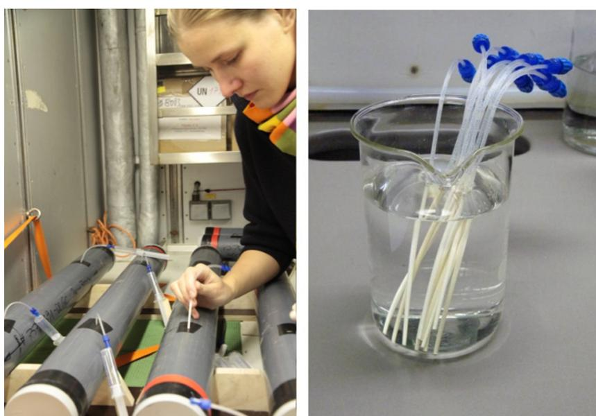
*Fig.13.1: Pore water extraction in 1 m core sections by means of rhizon in 50 cm core intervals (left side); Rhizons moistened in MilliQ water prior to be used (right side)*
