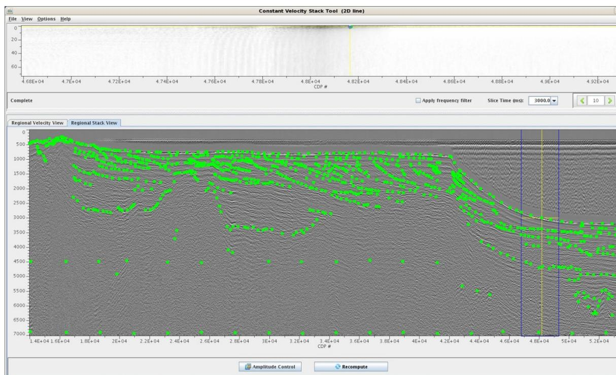
*Fig. 9.19: Java CVS tool – The bottom window shows the stack of the entire section with all velocity picks. Note the lateral coherency of picks of a certain reflector. The blue lines indicate the cdp window that is active for doing the velocity analysis. The top window shows the semblance result of the selected time slice.*
