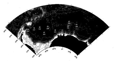
Fig. 9.1: Sound source array as currently installed. Numbers next to the dots indicate sound source labels and corresponding mooring numbers. Mooring 240 / sound source W3 will be recovered and redeployed during ANT-XXV/2.
