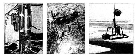
Fig. 9.1: Microprofiler (a), free falling lander system (b), and wire-driven profiler (c)
