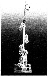
Fig. 9.3: Bottom water sampler
