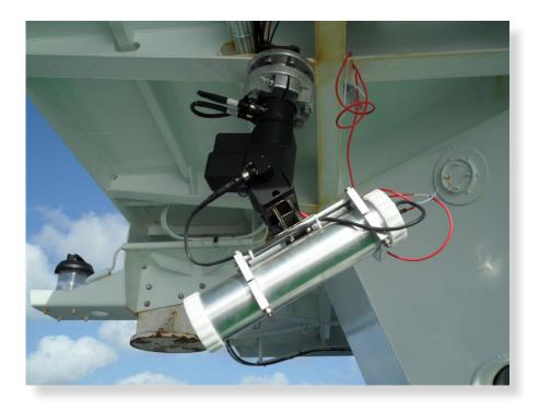
Fig. 13.1: The high-resolution camera in its metal housing mounted to the Pan-Tilt-Unit (PTU, black) installed on Polarstern's crow's nest.
