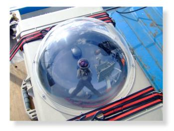
Fig. 3.3.2: Close-up photograph of the full-sky polarimetric cloud detector. (photo by András Barta)
