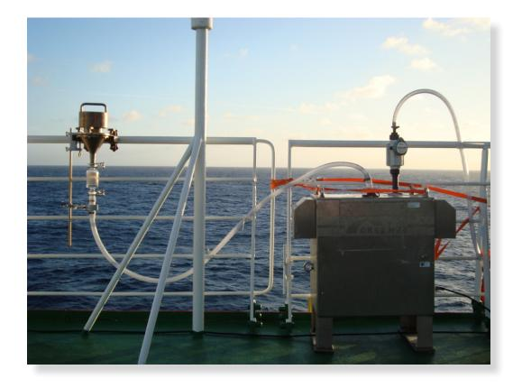
Fig. 9.1: High volume air sampling operated aboard F/V Polarstern during ANT-XXVII-1 (photo by Jasmin Schuster).
