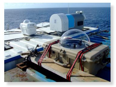
Fig. 3.3.1: Full-sky polarimetric cloud detector (right) in the vicinity of the full-sky photometric cloud detector of the OCEANET team (left) on top of the OCEANET container.(photo by András Barta)
