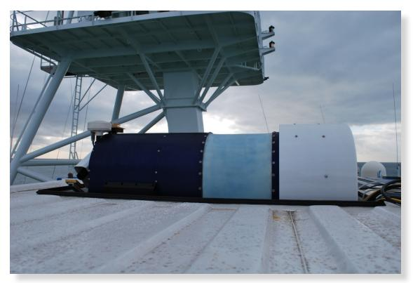
Fig. 3.1.1: Microwave radiometer HATPRO on the top of the OCEANET-atmosphere observatory (photo by Karl Bumke).
