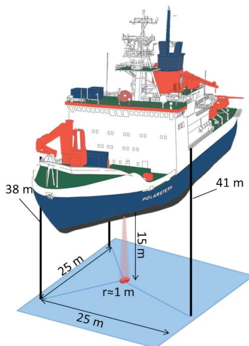
Fig. 3.8.1: Location of deployment of the three underwater winches or 'plumbines' (black vertical lines), respectively, and plain of calibration (blue area). Blue thin lines represent the lines connected to small calibration sphere. The red circle marks the sound beam area (radius ca. 1 m) in 15 m depth underneath the ship.
