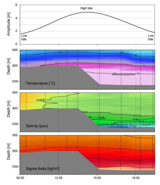
*Figure 9:* CTD casts collected with MUC between 09:00 a.m. and 19:30 p.m. (UTC) in relation to the tidal cycle from St. Mary's, Isles of Scilly, England. All presented parameters follow the tidal cycle at ~800 m water depth with an amplitude of ~50 m.
