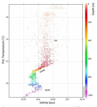
**Figure 8:** Potential temperatur-salinity-depth plot of CTD cast 2-7 indicating the different water masses: SW = Surface Water (0-100 m), ENAW = Eastern North Atlantic Water (100-750 m), MOW = Mediterranean Outflow Water (below 750 m).
