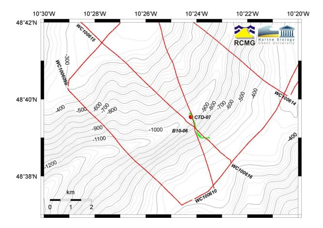
*Figure 5:* Detailed view on the observations made during ST1017b within the westernmost canyon; seismic profiles (red line), MUC station (yellow star), CTD cast (red circle) and ROV track (green).
