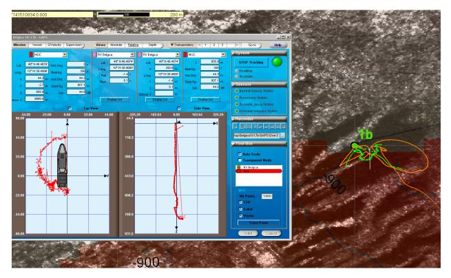
**Figure 7:** Screenshot from the combined OFOP and IXSEA GAPS navigation software, showing, in the background, the track of R/V Belgica (orange) and ROV Genesis (green). The IXSEA GAPS software shows the location of the ROV with respect to R/V Belgica in both horizontal as vertical plains. This screen was available both on the ROV container as on the bridge of R/V Belgica, assisting the navigation officers.
