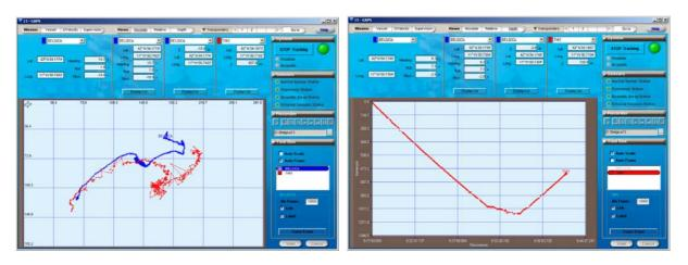
*Figure 7:* Screenshots of the GAPS software used to obtain a more accurate position of the boxcore: the absolute position of the ship and the boxcore (left) and the depth (right).
