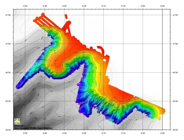
data editing. Various grid-sizes were used (30 to 5m) depending on the displayed map size and water depth.
