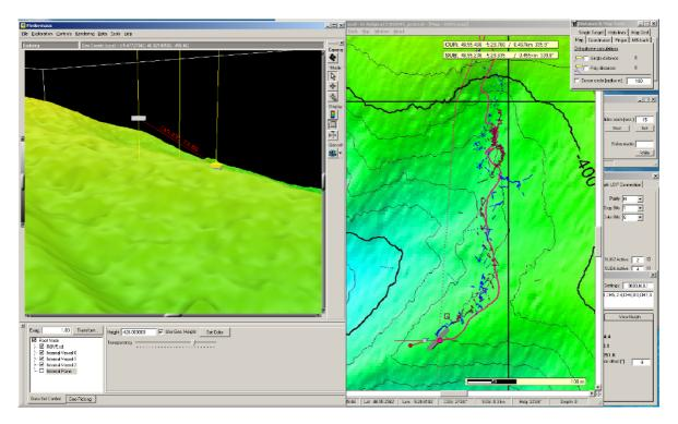
Figure 5: Screenshot of the 3D Fledermaus (grey box = TMS and yellow box = ROV) (left) and the OFOP software (right) for navigation during the ROV deployments.
