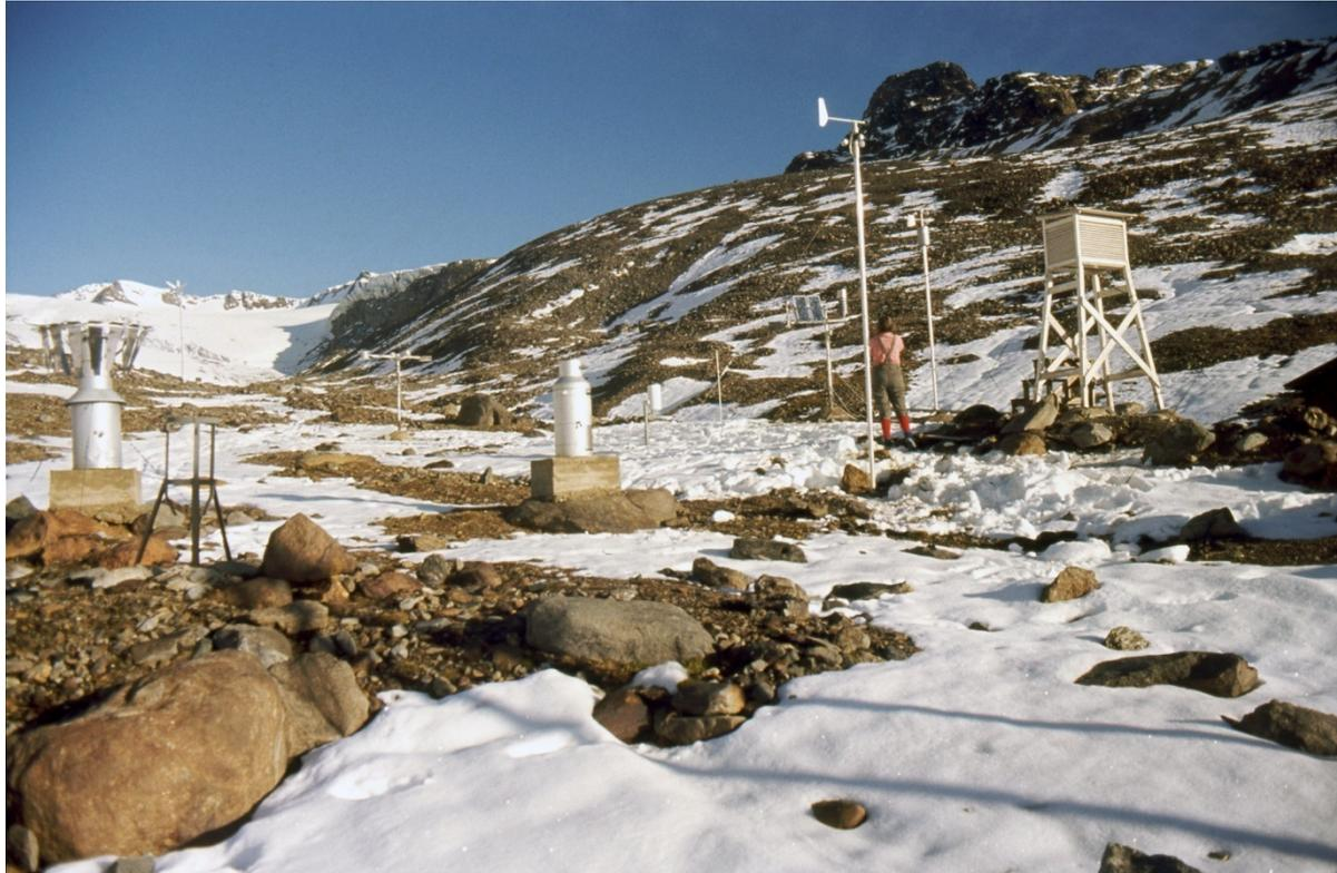
Fig. 1: Meteorological site of the Vernagtbach station; from left to right: Fuess precipitation gauge with wind shield, radiation instruments, Belfort precipitation gauge, Gertsch tipping bucket, solar panel and hair hygrometer, Thies anemometer, Wölfle anemometer, Stevenson screen with air temperature and BTW long-term thermo- and hygrograph inside. The photograph was taken by Markus Weber in October 1984.
