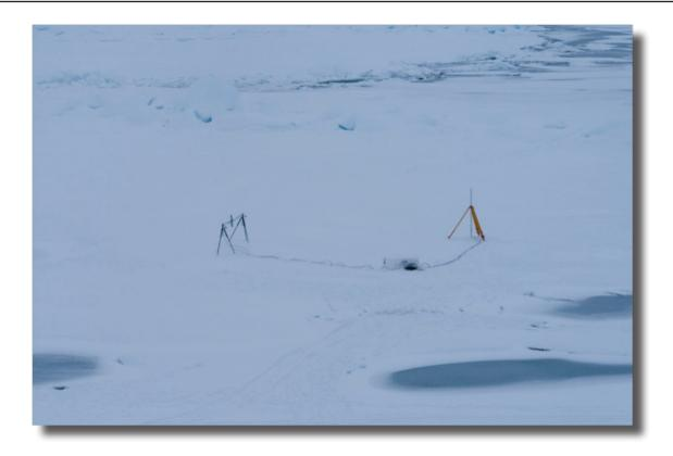
Fig. 3.12: Photograph of the radiation station. Two sensors are mounted above the surface for albedo measurements (left rack), one mounted on an I-arm held by the yellow stand, and two hanging under the ice at the position of the I-arm. Station on September 5 (78-238).
