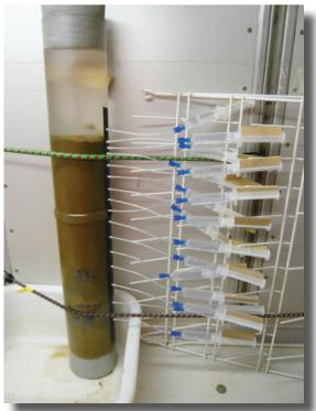
Fig. 8.7: Pore water sampling of a MUC
