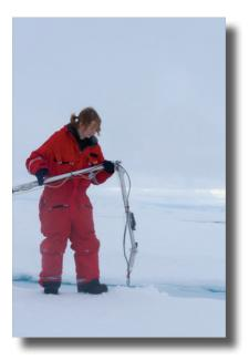
Fig. 3.13: Photograph of underice radiation measurements using a foldable holder, so called I-arm. Station on August 29 (78-227).
