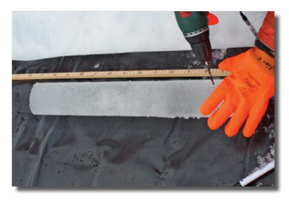
Fig. 3.18: Drilling of small holes in a sea ice core in preparation for temperature measurements every 10 cm
