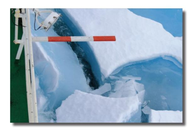
Fig. 3.27: Observation from the bridge: Ruler to obtain the thickness of tilted sea ice when the ship is breaking ice. This broken floe has a thickness of approximately one meter.
