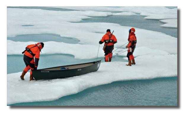
Fig. 3.23: Ground-based sea ice thickness survey with an EM31 Mk II (Geonics Limited). The instrument was towed over the sea ice in a canoo, which also allowed ice thickness measurements in melt ponds (Photo: Estelle Kilias).
