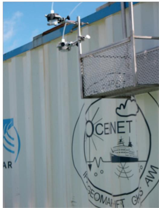
Fig. 8.1: Sampling inlets for the nitrite-coated filter sampler and continuous ozone monitor installed outside of the OCEANET container
