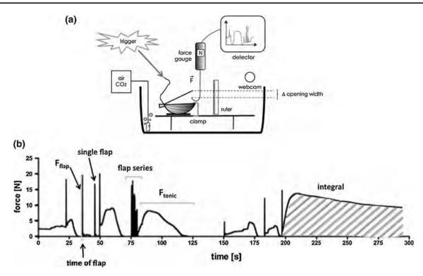
**Fig. 1** Scheme of clapping performance data collection on *P. maximus*. **a** Experimental set up for force measurements. **b** Example for force recording and visualization of clap force  $(F_{\text{clap}})$ , single
