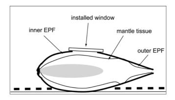
**Figure 1**: Sketch of prepared clam for microscopic pH measurements. The installed window allows to view into the inner EPF and onto the outer mantle epithelium (OME) of the mantle tissue. The connection of the mantle tissue with the shell (on the pallial line) separates the inner and the outer EPF. The animal was embedded in a thin sand layer (dashed line) for stability.
