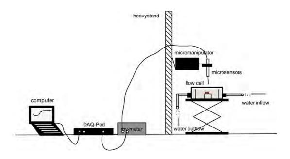
Figure 2: Microsensor set up.
