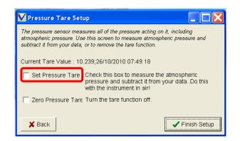
**Set pressure tare**: measures the pressure at sea level (atmosphere) and subtract this value from each subsequent pressure reading (recommended for profiling mode)
