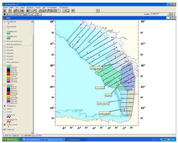
*Figure 1. Bay of Biscay map and PELGAS survey design. Blue lines: acoustic transects; red dots: trawl haul station; colored areas: post-stratification regions.*
