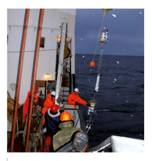
*Fig. 3.2: Deployment of a mooring in the Laptev Sea. For an entire year, the instruments register changes in currents, water temperature, and salinity due to sea ice formation and river water influx from the Lena River. (Photo: Heidi Kassens)*
