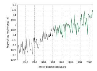
*Fig. 2.4: Regional average sea level for the German Bight determined with two different methods (mean approach 1843-2008 (black); EOF method 1924-2008 (green)) derived from 15 tide-gauges in the German Bight. The period 1843-1924 is only given for one tide-gauge, three additional time series exist for the period since 1900. (Graphic: HZG)*
