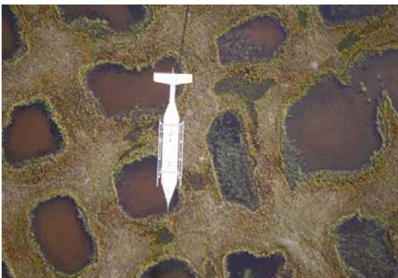
Fig. 3.4: The helicopter towed sensor "Helipod" during measurement of turbulent heat and CO<sub>2</sub> fluxes over the Siberian Lena Delta. (Photo: Torsten Sachs, GFZ)
