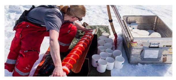
Figure 91: Preparation of sea-ice core for segmentation. Photo: Mario Hoppmann
