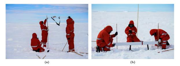
Figure 23: Calibration in (a) HCP and (b) VCP mode. Photos: Uwe Baltes
