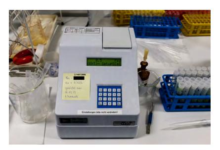
Figure 96: TD-700 Laboratory Fluorometer by Turner Designs. Photo: Mario Hoppmann
