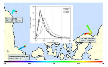
Flight tracks of laser scanner measurements in the Beaufort and Lincoln Sea. Colored dots indicate mean sea ice freeboard averaged over 10 km, the histogram shows the freeboard distribution of the respective regions for the profiles.
