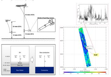
Left: Sketch of airborne sea ice thickness measurements with electromagnetic induction sounding based on 1D assumption: Electrical conductivity of sea ice negligible and level sea ice within footprint. Sea ice thickness is derived from the difference between sea ice/snow surface (detected by laser altimeter measurements) and the sea ice-ocean interface (derived from EM data).
