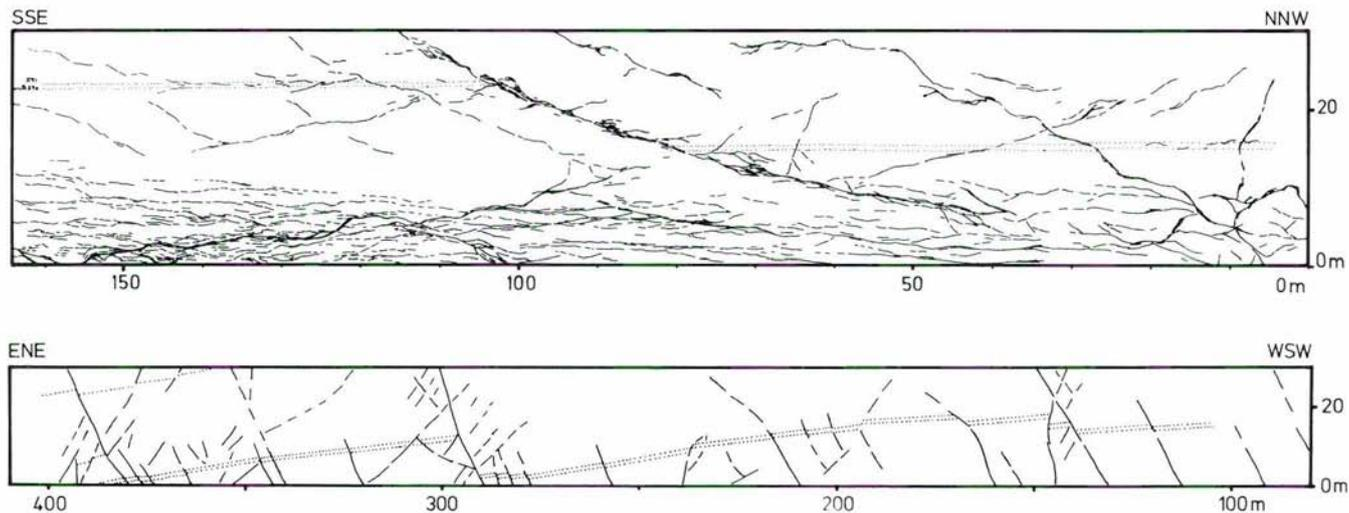
Fig. 2. Fracture mapping in the quarry Saturn. The W-wall section (above), subparallel to fault orientations, shows the detailed pattern and indicates a highly deformed rock complex. The S-wall section (below) perpendicular to the fault orientation shows the SW-ward downstepping of the tilted fault blocks.
