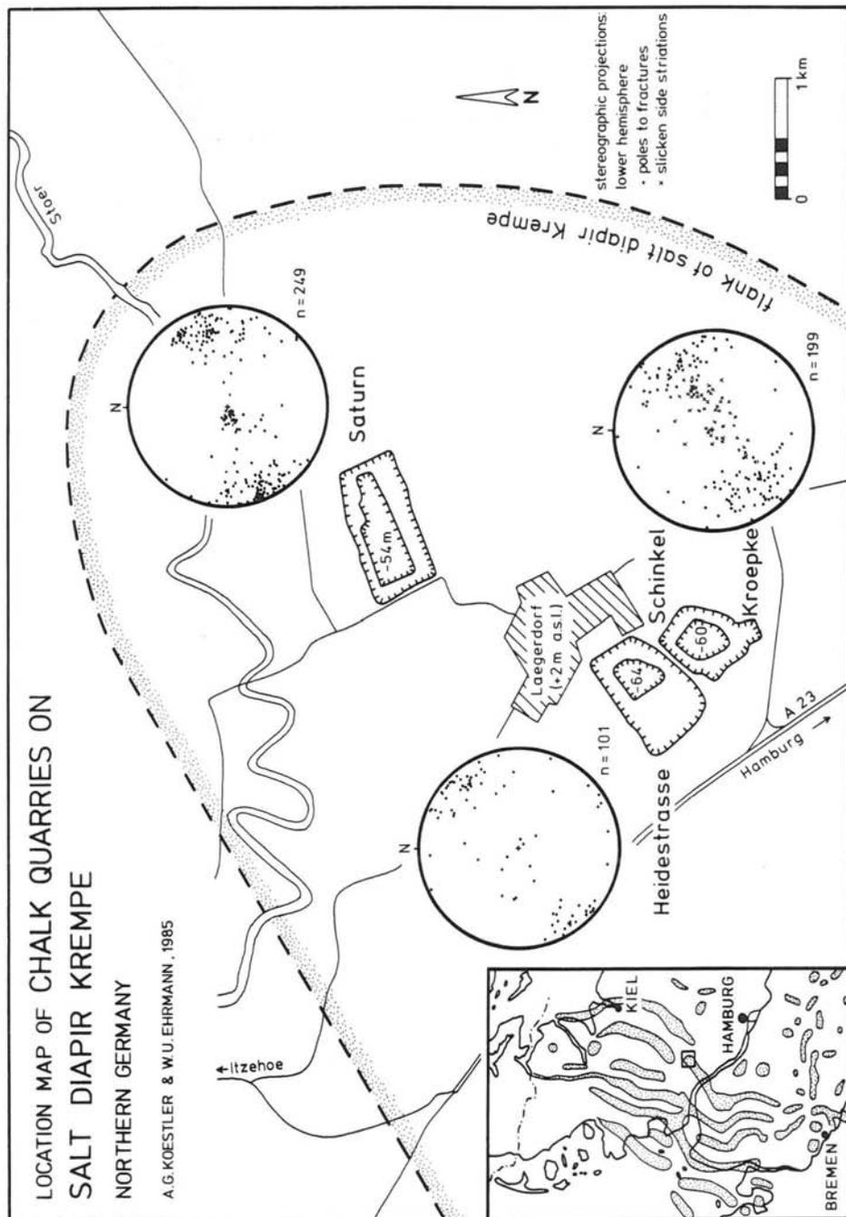
Fig. 1. Location map of the chalk quarries near Laegerdorf. The index map shows the salt ridge configuration of Northern Germany (from JARITZ 1973). The circles represent stereographic projections of fractures measured in the individual quarries.
