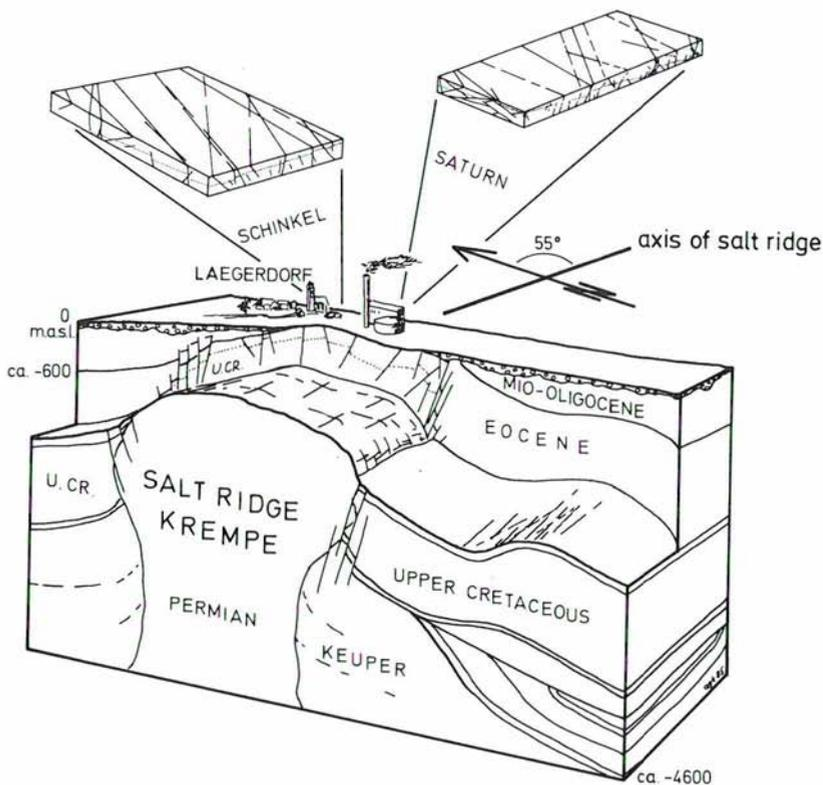
Fig. 5. Schematic block diagram of the tectonic situation of the quarries on salt ridge Krempe (geologic section redrawn from GRUBE 1955).
