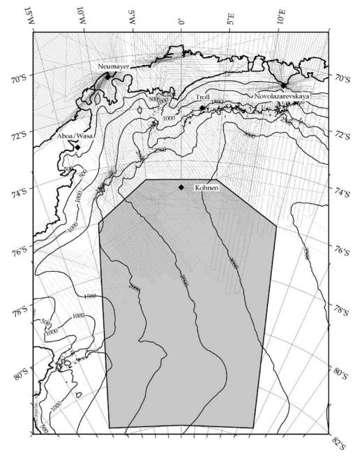
Figure 2-5: The proposed flights for WEGAS will be conducted in the grey shaded area south of KOHNEN. The line spacing will be 10 km, the orientation of the lines 0°. Test and calibration flights will be carried out in the grey shaded area around NEUMAYER STATION III The tracks of the earlier surveys VISA and WEGAS are shown as thin grey lines.
