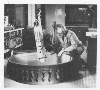
Testing of an instrument in the pressure tank prior to the deployment at sea (photo: E. Mempel)
