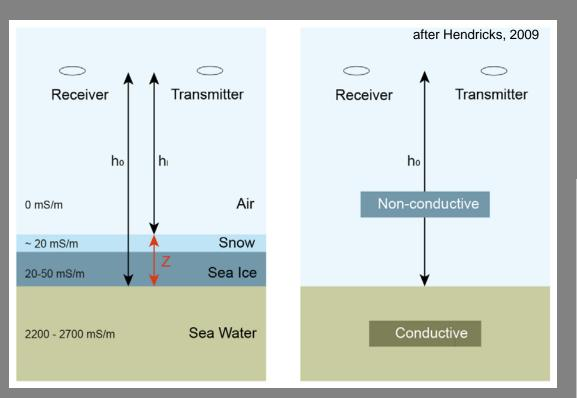
h<sub>I</sub> Measured with laser altimeter
