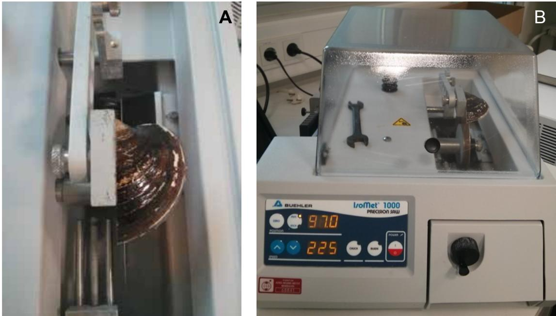
Fig. 6: Low-speed saw used for cutting bivalve shells on the line of strongest growth. (A) One shell of *A. islandica* is glued on a metal block with Crystalbond. (B) Shells were cut with a rotation speed of 225 rpm.
