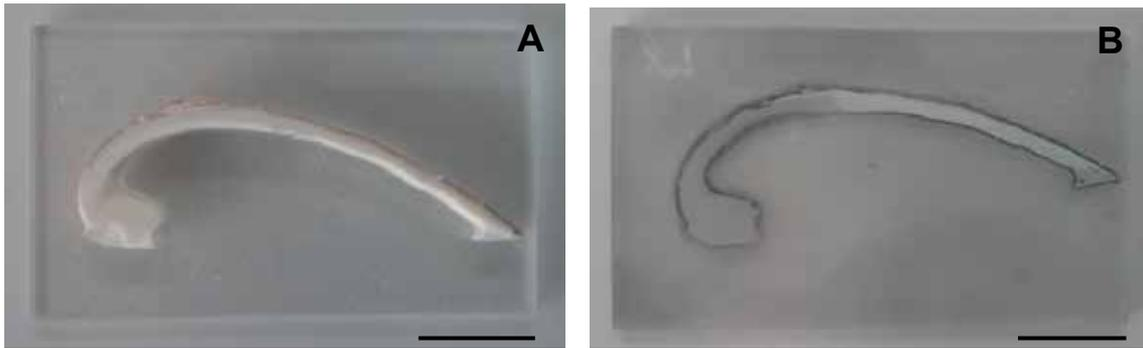
Fig. 9: (A) Cross-section of *A. islandica* is glued on a lapped glass-slide with EPO-TEK. (B) Lapped cross-section of *A. islandica* (shell-ID: 090928). Most parts of the shell material are lost and in the remaining shell material, there are no microincrements visible. The black line in both images illustrates scale of 1 cm.
