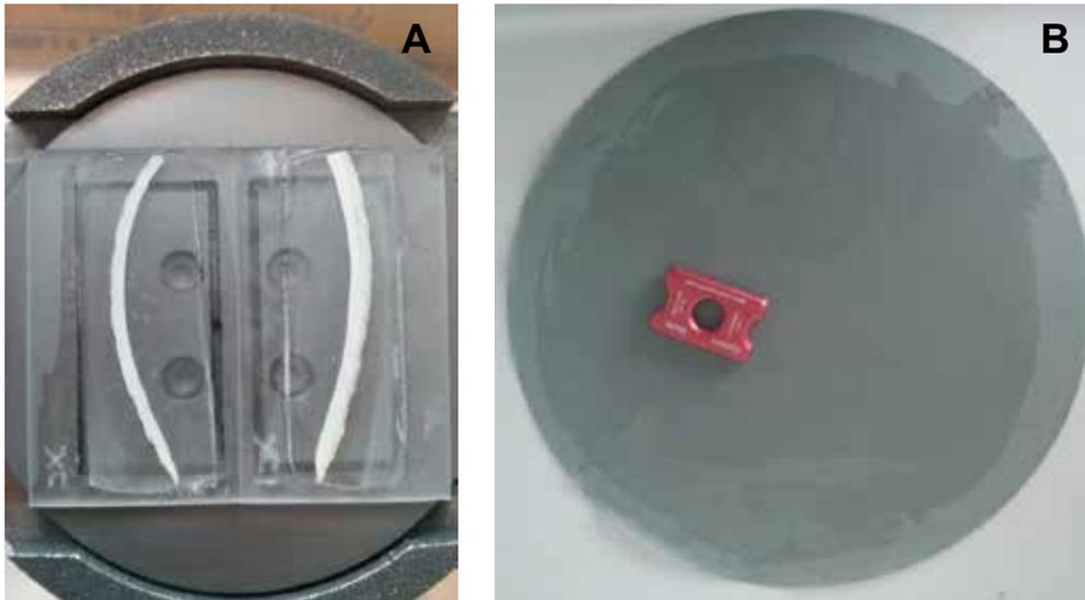
Fig. 8: (A) Bottom side of the supporting head of the lapping and polishing machine. The two thin-sections are cut down to 200  $\mu\text{m}$  and currently in the lapping process. (B) Sandpaper with different grain size is used to grind and polish the thin-sections. For this, glass-slides were mounted into the red holder and moved in irregularly circles over the sandpaper.
