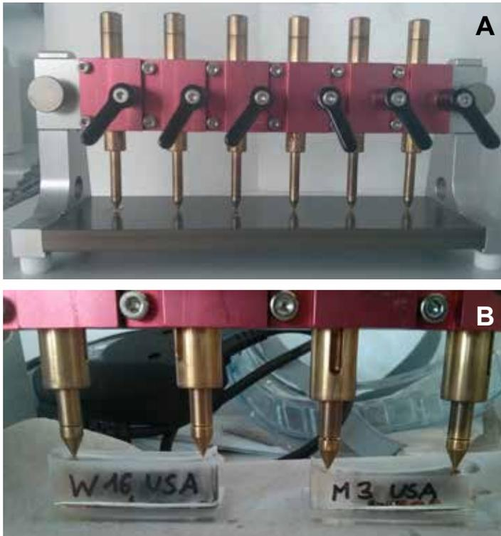
Fig. 7: (A) Special press gadget. (B) Bivalves with higher ontogenetic age are embedded in bigger aluminium rings and they were pressed to the glass-slides on two points.
