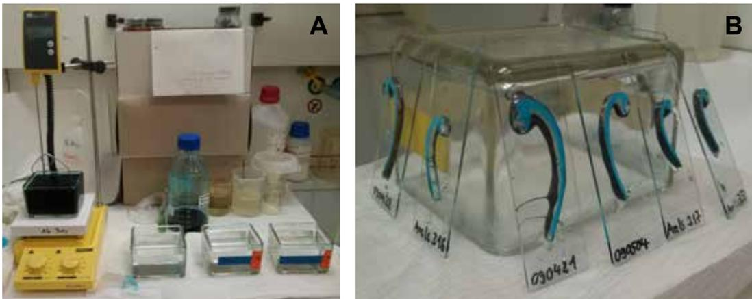
Fig. 12: (A) shows the necessary laboratory equipment and chemicals for dyeing thick-sections with Mutvei's solution. (B) Thick-sections dyed with Mutvei's solution. They are just air-
