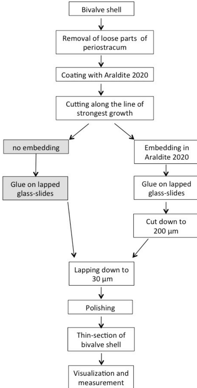
Fig. 1: Flow chart describing the preparation of thin-sections from bivalve shells. The grey-colored path has been tested, but finally considered unsuitable for the preparation of thin-sections.
