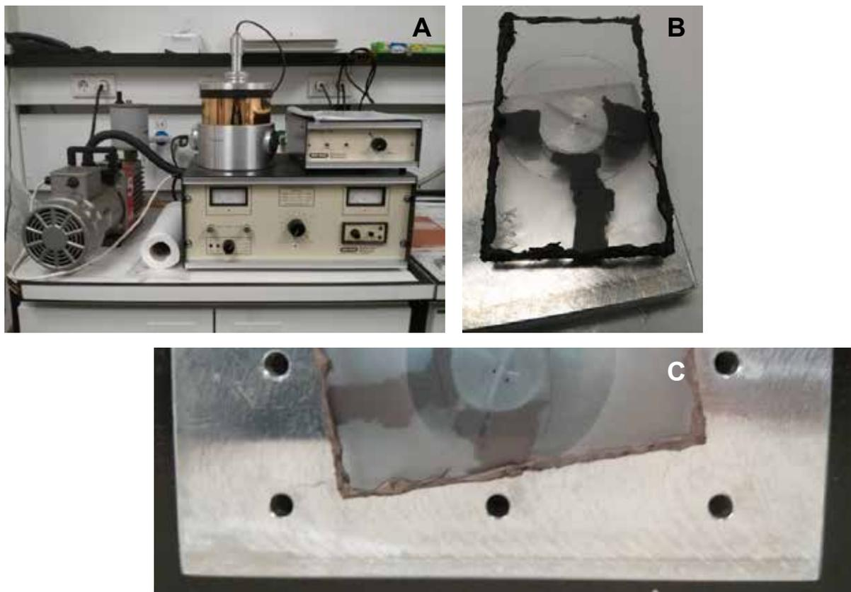
Fig. 11: (A) Sputtering machine. (B) Thin-section of *A. islandica* coated with Lite C. This preparation is necessary before the sample can be sputtered with gold. (C) Gold-sputtered thin-section.
