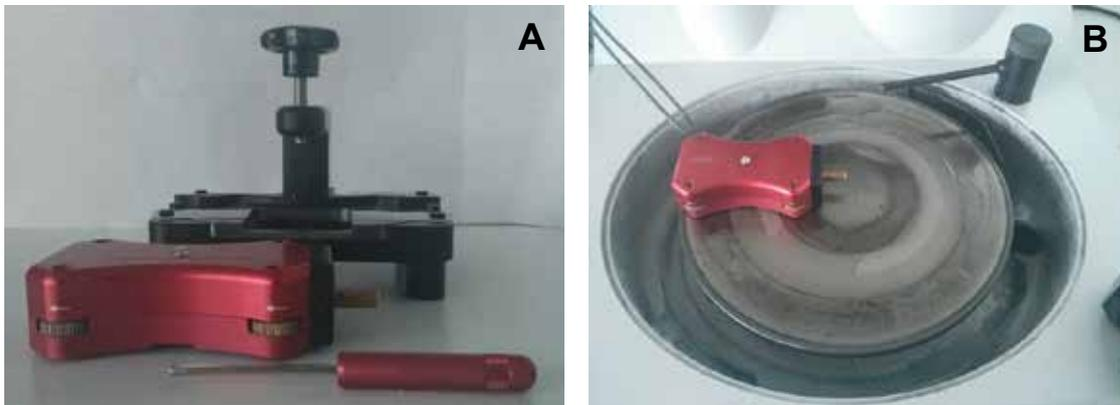
Fig. 10: ABELE-System, which has been used for grinding thin-sections. (A) Complete ABELE system components which are necessary to adjust the thickness. (B) The red glass-slide holder needs to be pressed onto the rotating grinding disc while a constant water flow wets the disc. Two different discs with different grain size 15  $\mu\text{m}$  and 10  $\mu\text{m}$  respectively have been used in this study.
