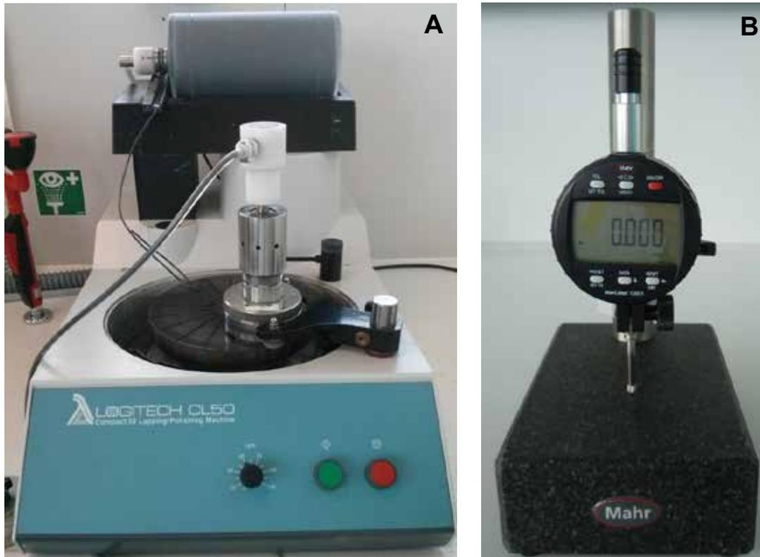
Fig. 5: (A) Lapping/ Polishing Machine and (B) Dial gauge.
