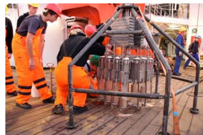
Successful recovery of the sediment surface with the MultiCorer, MUC (Photo: Thomas Ronge)
