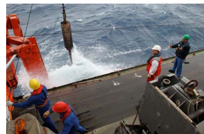
Operating the gravity corer during rough sea (Photo: Thomas Ronge)
