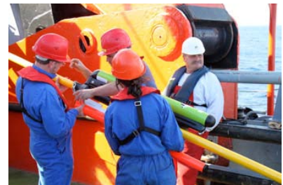
Fitting the stabilizer to the „Streamer“ (Photo: Thomas Ronge)
