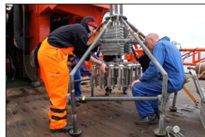
Setting up the Multicorer (MUC) for sampling the sediment surface (Photo: Thomas Ronge)
