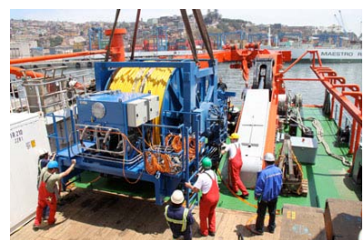
Installation of the seismic winch at the afterdeck (Photo: Thomas Ronge)
