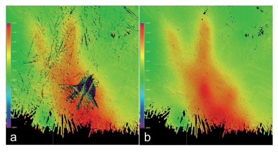
Fig. 12.1: Bathymetric data during heavy icebreaking activities (a) before and (b) after data cleaning
