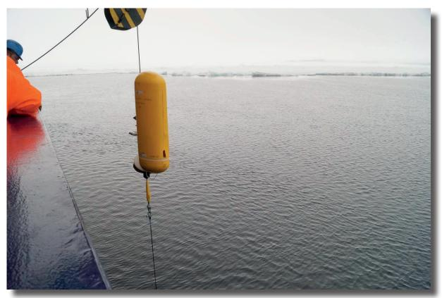
Fig. 8.3: Deployment MMP- profiler
