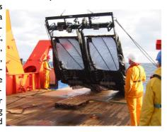
not allow for using towed gear, so we started with several CTD/rosette casts. On the following day, the weather and sea conditions improved considerably, and one  $10~\text{m}^2$ -MOCNESS haul (down to 1000~m) and two hauls with the  $1~\text{m}^2$ -double-MOCNESS (down to 4170~m) could be performed.
