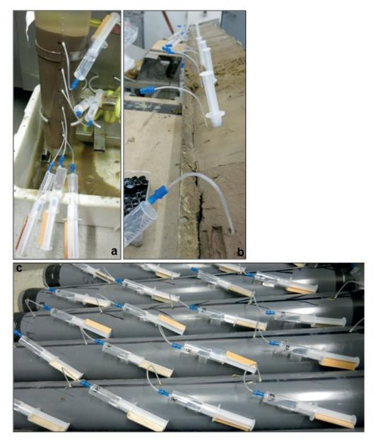
*Fig.* 10.9.1: Pore water sampling; a: Multi-corer tube (5 cm intervals); b: Box core sediment (20 cm intervals); c: Gravity corer segments (20 cm intervals)
