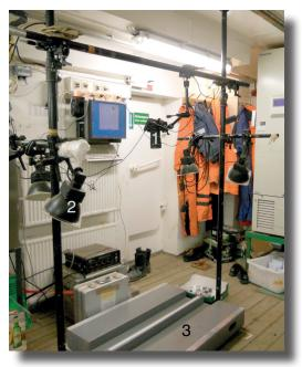
Fig. 10.1.4: Photographic system that was used on board. 1: Camera (Nikon D700), 2: Flash Lights, 3: Core table
