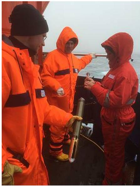
Fig. 6: The UCTD probe and its connection to the thin Kevlar line are inspected on the stern of the ship between test profiles on the transit to the first mooring location. Photo R. Stein/AWI
