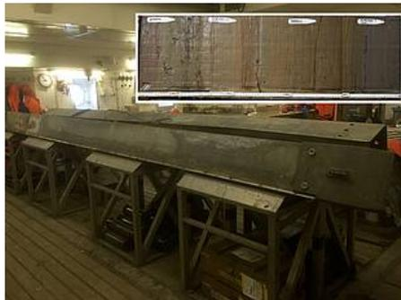
Fig. 3: Kastenlot cores not opened yet (main photo). In the top a one-meter section of the opened kastenlot core. (Photo R. Stein/AWI)
