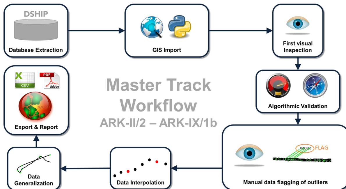
**Figure 4: Workflow of master track data processing (ARK-II/2 – ARK-IX/1b)**
