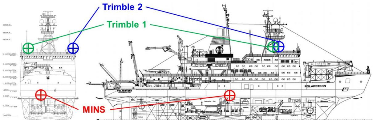
**Figure 7: Locations of positioning sensors on RV Polarstern**
