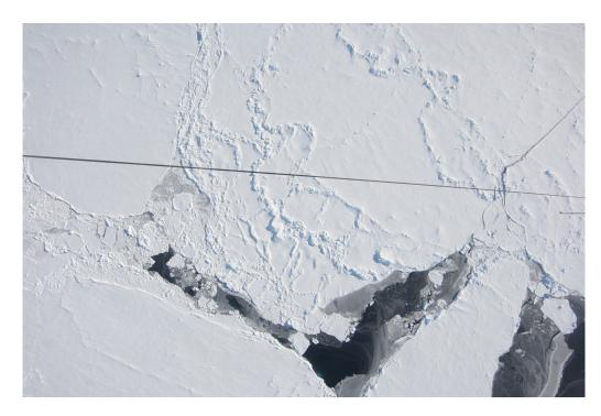
Figure 4.8: This photograph was taken with the camera system during PAMARCMiP'11 on 14.03. and it shows a very typical sea-ice surface with parts of open water, new ice and snow covered thick ice floes. The dark line crossing the image is the towing cable of the EM-Bird.
