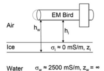
Figure 4.13: The EM-Bird system measures the distance  $h_w$  above the ice-water interface as the field strength of a secondary EM field and the distance  $h_i$  above the ice with a laser altimeter. Difference of distances gives the ice thickness  $z_i$ . Here,  $\sigma$  denotes the conductivity of the media. From [Haas et al., 2009]
