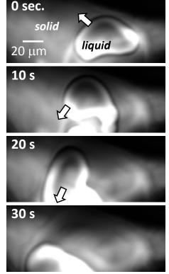
Figure 1. LCM-DIM images of liquid layers on an ice basal face at
