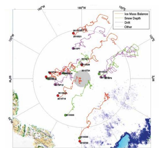
Snow buoys (green lines) contribute to a network of autonomous platforms in the Arctic (deployed in autumn 2016). (Figure: www.seaiceportal.de)
