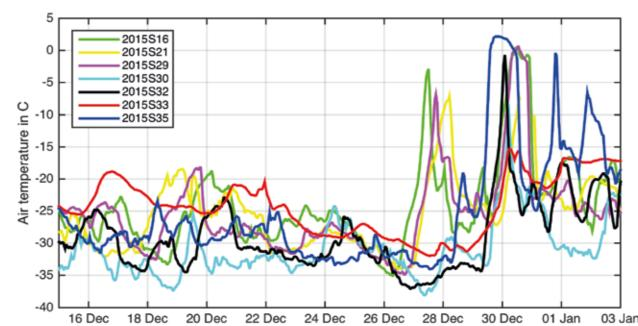
Air temperature measured by snow buoys in the Central Arctic in December 2015.
