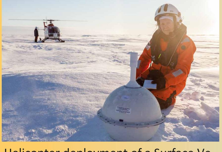
Helicopter deployment of a Surface Velocity Profiler.
