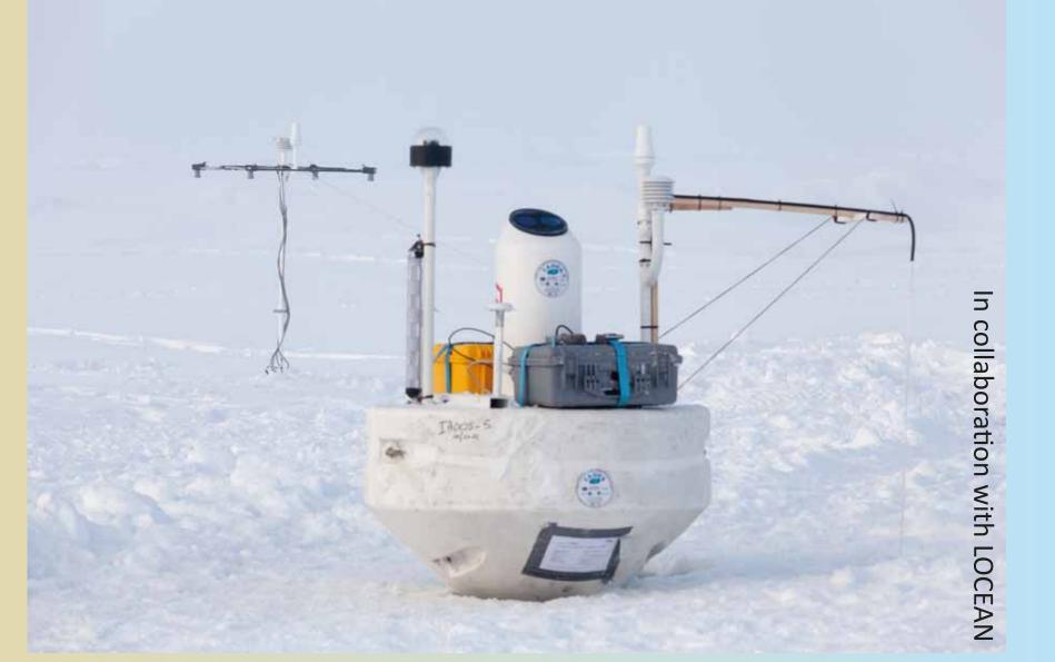
Ice-Atmosphere-Arctic Ocean Observing System (IAOOS) with upper ocean profiler, LIDAR and ice mass balance buoy.
