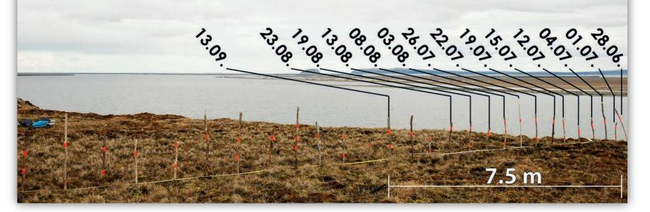
Time-lapse camera setup at the test site. We installed 29 wooden markers every 50 cm perpendicular to the cliff top and a Brinno TLC200 Pro time lapse camera viewing from South to North. Pictures were taken every four hours from 28.06.2015 to 13.09.2015. In that period 15 markers were eroded, equaling 7.5-m of cliff top retreat.
