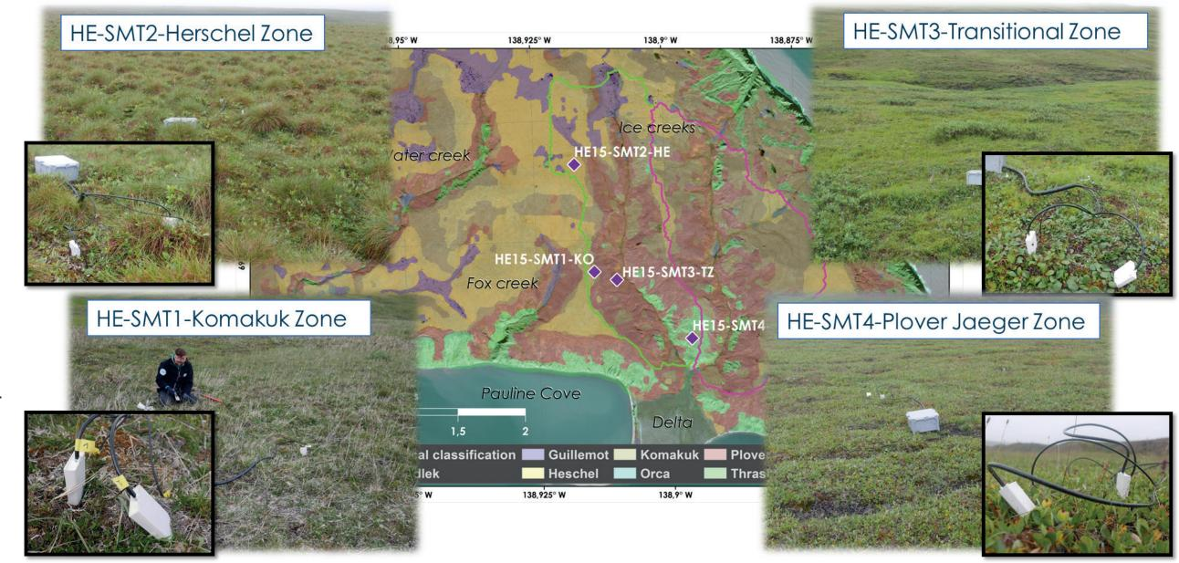
Four stations measuring soil moisture and temperature close to the surface were installed in July 2015 in four different landscape units to compare the influence of snow on the soil moisture dynamic. Each stations has two soil moisture and temperature sensors each that are installed vertically and diagonal. Animal attacks of the stations are a risk.
