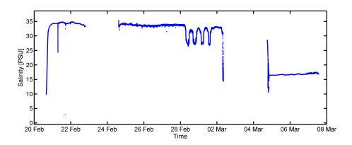
Figure 6: Salinity after speed filter.
