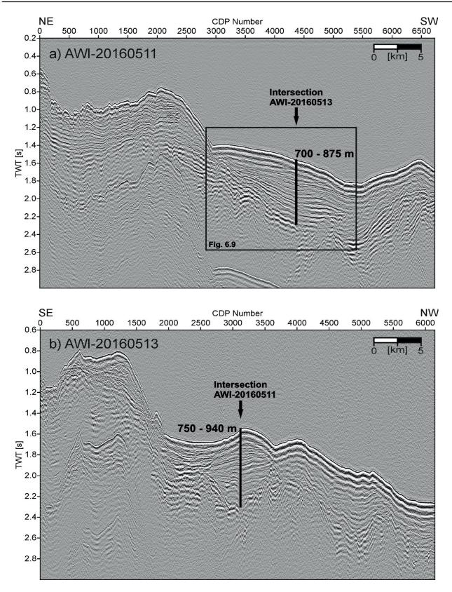
Fig. 6.3.7: Multi-channel reflection sections of potential IODP site 2. a) Seismic line AWI-20160511 in NE-SW direction. b) Seismic line AWI-20160513 in SE-NW direction. The seismograms are shown as time-section with two-way traveltime (TWT) at y-axis. At the x-axis CMP numbers are shown. Depth values are estimated with a sound velocity of 2000 - 2500 m/s.
