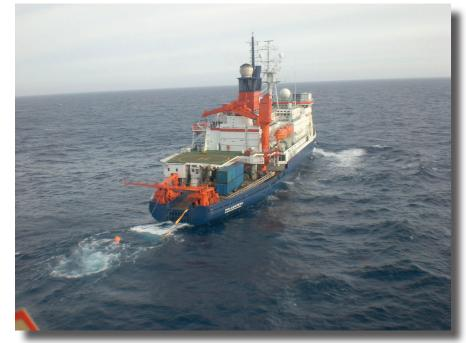
Fig. 6.3.4: Photo of RV Polarstern with the towed airgun and 600 m multi-channel streamer (Photo:Sascha Plewe (IOW))
