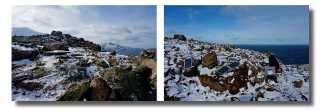
Fig. 4.4.4: Installation of the GPS equipment at the sites ELE1. The left photography shows mounted GPS antenna on the existing GAP marker from 1995. The right photography shows the solar-panels (left) for power supply of the receiver and the Zarges aluminium box (right) to protect the receiver and battery.
