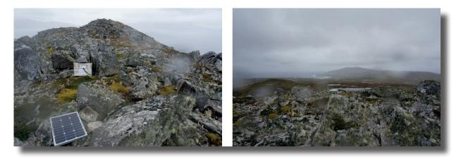
Fig. 4.4.5: Installation of the GPS equipment at the sites HORN. The left photography shows a solar panel and the aluminum box (the middle ground). The right photo shows the mounted GNSS antenna.
