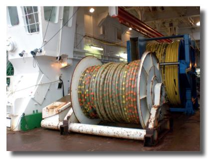
Fig. 6.3.3: The 600 m long analogue streamer (front) (Type PRAKLA) (Photo: Sascha Plewe (IOW))
