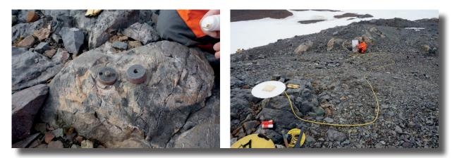
Fig. 4.4.3: Installation of the GPS equipment at the sites PRA1. The left photography shows the existing GAP (Geodetic Antarctic Project) marker from 1995. The right photo shows the mounted GPS antenna in the left foreground.
