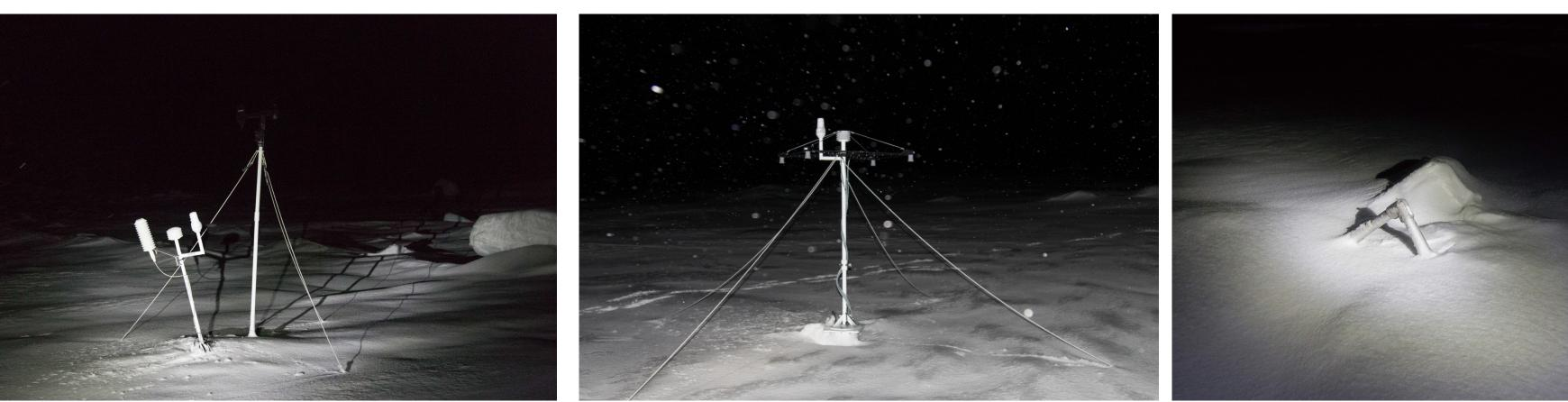
The Polar Atmospheric Weather Station (PAWS) was found in good condition. The slightly tilted instruments could be easily recovered.
