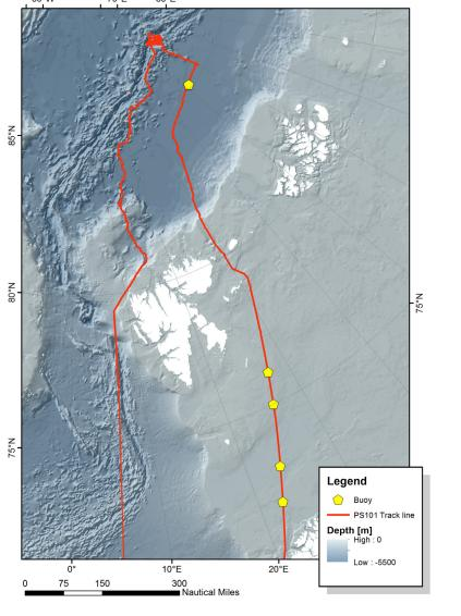
In total we deployed 8 surface velocity profiler (SVP) buoys, 8 GPS trackers, 5 Snow Buoys, 4 thermistorstring Ice-mass-balance buoys and two ITBOB prototypes including a solar-radiation package, as well as a triplet fluorometer and an oxygen optode underneath the sea-ice.
