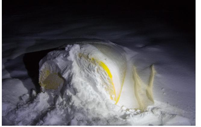
ITP93 had fallen over into an adjacent melt-pond. However it was still able to send data while being partly snow covered.
