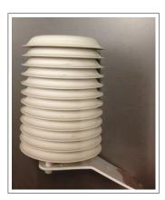
Figure 2: Combined air temperature and humidity sensor
