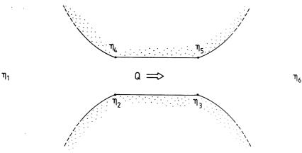
**Figure 2** The sea level ( $\eta$ ) at various positions in and outside a strait with flow rate Q = VHW
