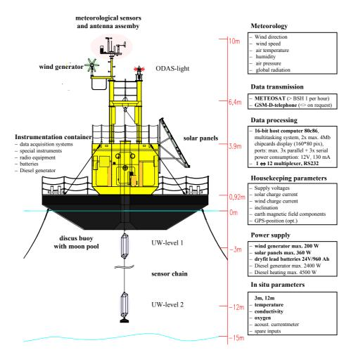
Figure 3 Discus Buoy at ODER BANK for monitoring of the exchange processes between the Pomeranian Bay and the Arkona Basin
