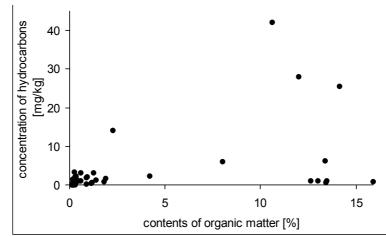
Figure 4 The hydrocarbon concentrations in the South baltic sediments as a function of their organic matter contents.
