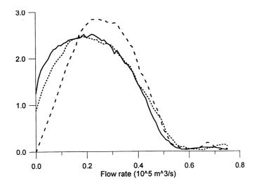
Figure 4 The probability density function of the absolute flow rate, p(|Q|), for the observed flow rate (solid line), the flow rate according to the quadratic model (dashed line) and according to the combined model (dotted line)
