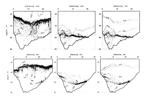
**Figure 5** Temperature, salinity, and potential density anomaly vs. distance and depth for transects across the Stolpe furrow (September 1994, 33rd cruise of r/v "Professor Shtockman"). Top panels are from transect 2b, and bottom panels are from transect 3b.
