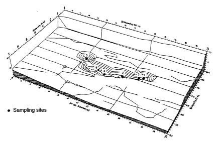
Figure 3 Bottom bathymetry of the Kuznica A pit (1990).
