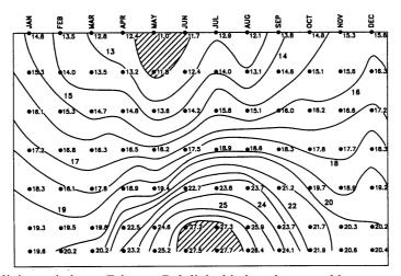
Figure 4 The yearly salinity variation at Fehmarn Belt lightship based on monthly average conditions presented in Lange *et al.* (1991). The hatching shows the minimum and maximum salinity.
