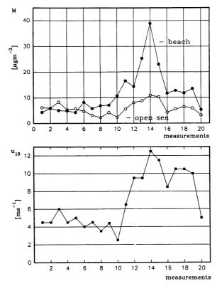
Figure 1 The comparison of the mass concentration of sea salt for the open sea and the beach as a function of wind speed.
