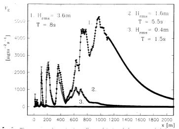
Figure 3 The aerosol emission flux obtained from model for three boundary conditions for the sea bottom profile in Lubiatowo
