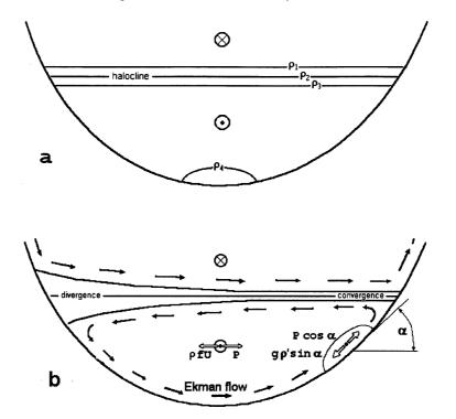
Figure 7 An explanation of the fan-like shape of isopycnals and northward displacement of the densest water pool from the deepest connection observed on transects across the Stolpe Furrow.
