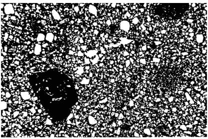
**Figure 2** Silty till (gl  $Q_{III}$ ) with admixture of rounded fine sand grains and gravel size black angular limestone fragments. The clayey matrix (dark) contains dispersed quartz, carbonates, feldspars and other mineral debris. The Baltic sea, Sambian-Kura high, bore hole 12, depth 5.5m. Photomicrograph of the thin section in transmitted light, magn. 40 X.
