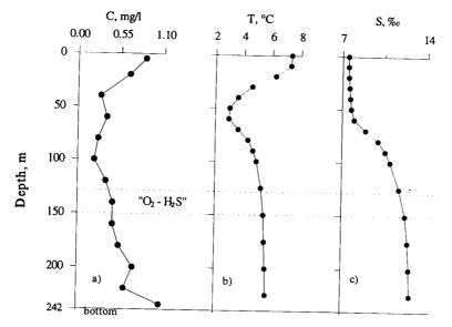
Figure 3 Vertical profile of suspension concentration in the Gotland Deep. Dotted lines show the geochemical " $O_2$ -H<sub>2</sub>S" barrier.
