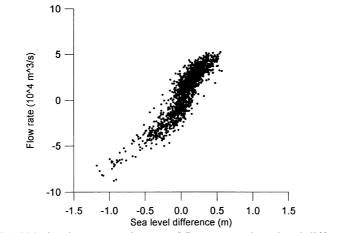
Figure 3 1802 simultaneous estimates of flow rate and sea level difference
