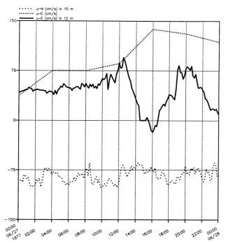
Figure 9 Current speed towards N at station 532 at 10m depth in Langelands Belt, and towards E at station 528 at 12m depth and at Fehmarn Belt lightship.
