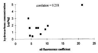
Figure 5 Correlation of the fluorescence coefficient and real concentration of hydrocarbons in water
