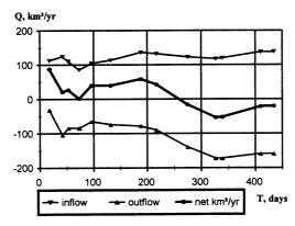
Figure 4 Evolution of the estimates of total in- and outflows and net exchanges depending on the lengthening of the direct measurements series in 1993–95
