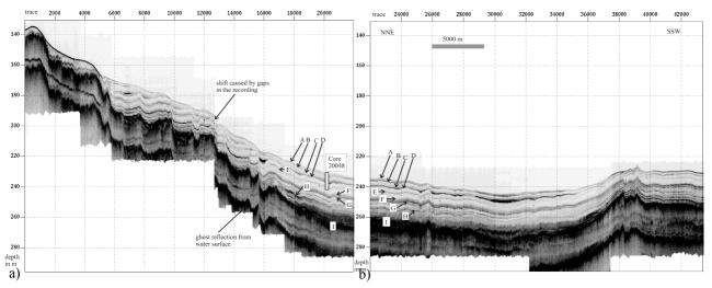
Figure 3 Acoustic image of Gotland Basin sediments—longitudinal section a) GeoChirp line 940830 northern part b) GeoChirp line 940830 southern part
