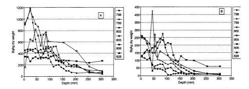
Figure 4 Radiometric profiles of sediment cores from the Gotland Basin. For location of sampling position see Figure 1. A) Depth profiles of supported <sup>210</sup>Pb activities.
