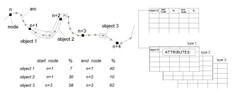
Figure 1 The dynamic segmentation data model
