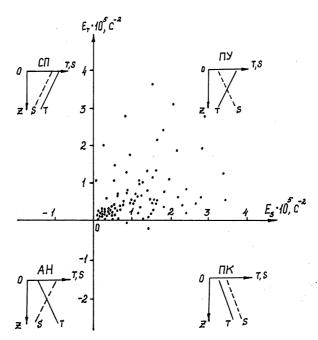
Figure 4 Types of thermohaline conditions characterising stratification (K. Ferorov's diagram) obtained from the measurements at stations of the polygon. C-solt fingers-like, Y-complete stability, K-layer-to-layer convection, AH- complete non-stability.  $E_T$  and  $E_S$  are temperature and salinity stability components.
