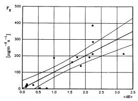
Figure 2 the emission flux of aerosol as a function of dissipation of wave energy to the power of 3/4
