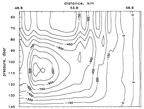
Figure 10 Geostrophic flow function vs. pressure and distance for a fragment of the A–B transect including the cyclone and its northern periphery
