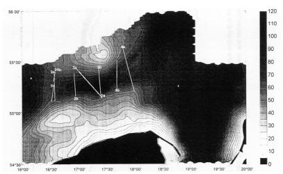
Figure 2 Detailed bathymetry of the Stolpe Furrow. 1a–4a are the PS-29 CDT transects (06–14.04.93) and 01b/1b–4b are the PS-33 transects (22–23.09.94)
