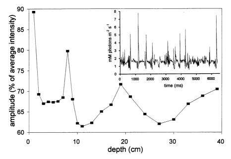
Figure 3 Depth profile of wave focusing effects in the DZBK near Zingst. The average amplitude of the wave-focusing effect is plotted as a percentage of the average irradiance. Measurements were made on 2.9.1995 between 10.45 and 15.15 with 8/8 thin stratus cloud cover. Shown in the insert is an example of a single measurement at a depth of 1 cm at the same station but with cloudless conditions (29.8.1995).
