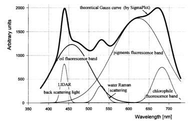
Figure 4 Calculated LIDAR fluorescent spectrum and theoretical fluorescent bands
