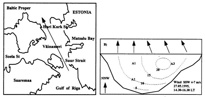
**Figure 1** The Väinameri area and the cross-section of the Suur Strait; current velocities in cms<sup>-1</sup>. AI, A2 and A3 mark the positions of the mooring stations.
