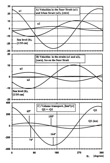
Figure 2 Dependence of velocities and volume transports in the Suur Strait and the Irben Strait on the wind direction ( $\phi$ , module=7ms<sup>-1</sup>) and on existence of ice in the Suur Strait area.  $Q_1 = H_1 = H_2 = 0$ .
