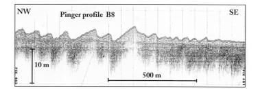
Figure 3 Pinger profile (B8) of sandwaves in the western part of Fehmarn Belt. Location indicated on Figure 1.
