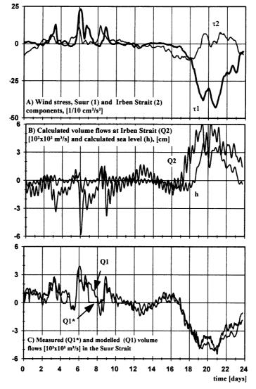
Figure 5 Comparison of the modelled and measured velocities in the Suur Strait (C) and some other modelled values (B) in the realistic external forcings (A). Note the malfunction (entangling) of the measuring equipment on the 8th day ( $Q_1^*$  in C).
