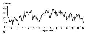
Figure 13 Current measurements with the Pettersson current meter in the Jutland current in August 1913 at 80 m depth. Component towards ENE.
