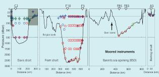
Fig. 1. Moored instrument locations during 2005-2006: Microcats (blue), RCMs (red), ADCPs (green). BI1-BI4 & WG1-WG4 in Davis Strait have not been analysed yet, and shaded in grey.
