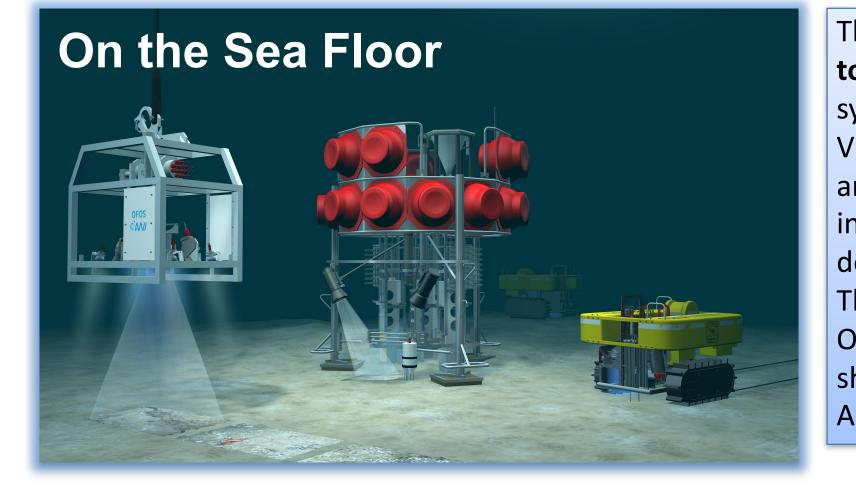
The modular benthic observatory consists of a towed camera system (OFOS), a benthic lander system and an **autonomous crawler (TRAMPER).** Visual observations, biogeochemical flux studies and ecological experiments give long term information on so far unknown processes at the deep seabed.
