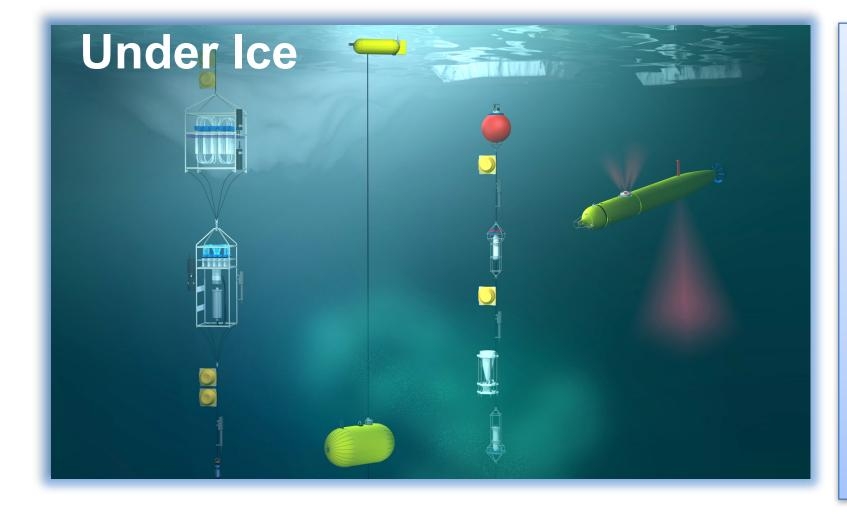
An innovative mooring concept studies the interplay between physical and biogeochemical processes and their effect on the food web: the mooring concept consists of a near surface mooring with water and sediment samplers and multiple biogeochemical sensor suites, a novel profiling winch unit (SWIPS), and a traditional mooring with sediment samplers and sensor suites.
