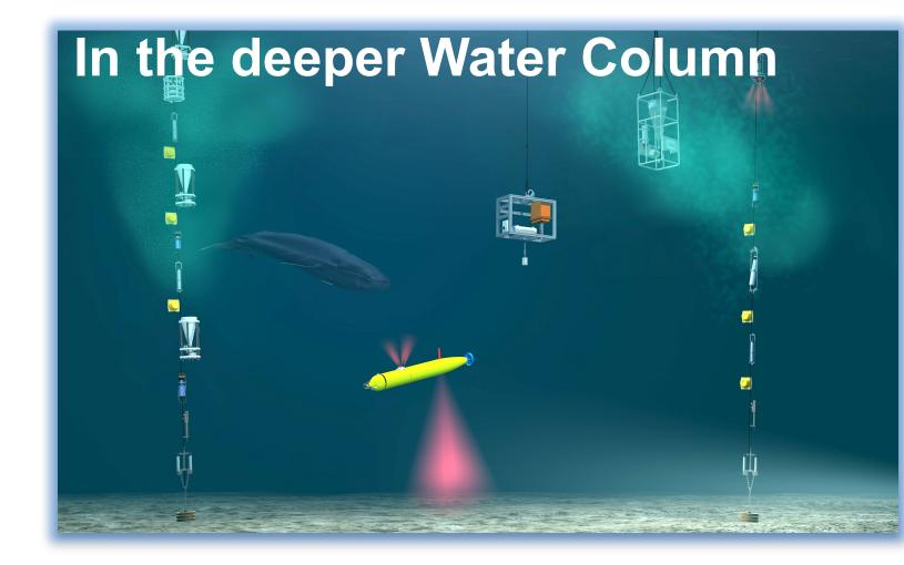
Multidisciplinary techniques are combined to study particle biogeochemistry, zooplankton ecology, marine mammals, and the physical and environmental characteristics: Moored BioOptical Platforms are completed by ship based particle cameras and traditional traps.
