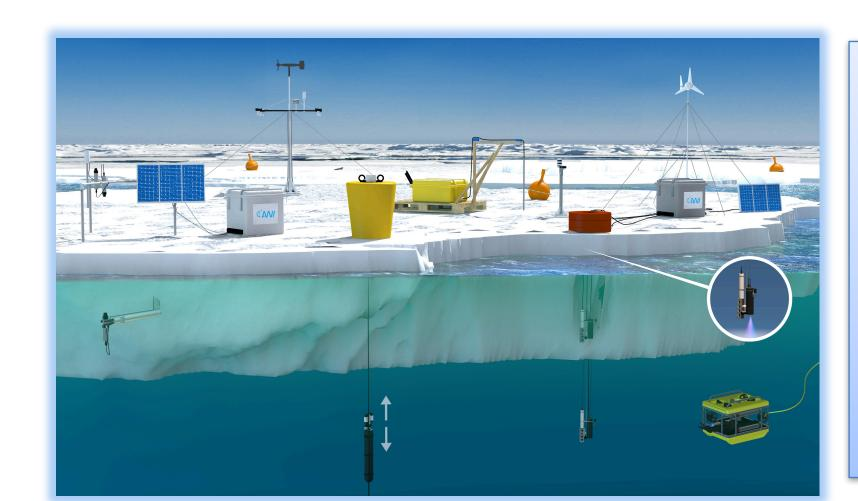
Ice buoys and ice-tethered platforms installed on ice floes in the central Arctic Ocean measure solar radiation, albedo, snow height, ice thickness, temperature, and algal activity. The data are delivered year round in partly near real time. The AWI sea ice buoy network is part of an international effort.
