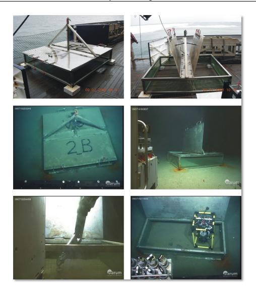
Fig. 2.1: Cages for the starvation experiment on board Polarstern (top) and at the deep seafloor (middle); sediment sampling and microprofiler measurements during Polarstern expedition ARK-XXIV/2 in summer 2009 (bottom)
