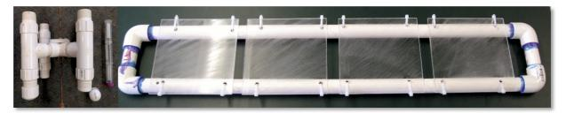
Fig. 2.5. Embedded funnel larval trap design (left side) and settlement plates (right side)
