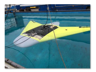
Fig. 7.1: The underwater glider being weight balanced in the test basin of MARUM
