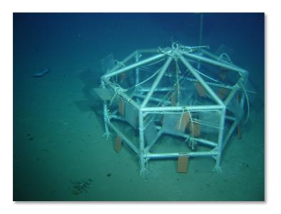
Fig. 2.6: Metal frame with different kinds of hard substrates deployed in 1999 at the central HAUSGARTEN site HG-IV
