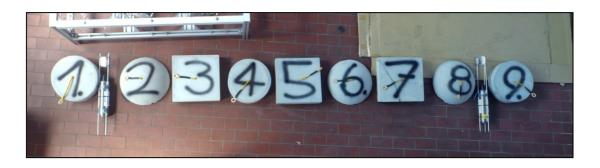
Fig. 2.3: Artificial dropstones and cylindrical homer beacons for tracking the stones at the deep seafloor laid out in a workshop before shipment
