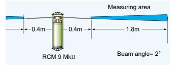
The instrument can operate continuously or in eight intervals from 1 to 120 minutes. At 60-minute recording interval the operating time is more than two years.
