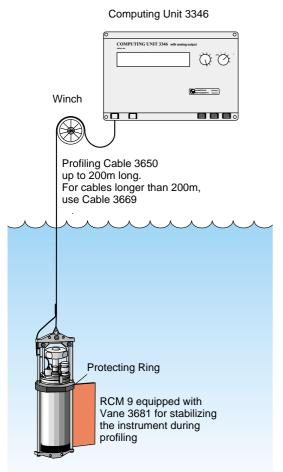
and as RS232 output for a PC. To stabilize the RCM9 during profiling, the mooring frame is equipped with Vane 3681. The response time (63%) is 12 seconds for the temperature sensor and one minute for the oxygen sensor. Data can be stored internally and read after retrieval if an ordinary mooring line is used.
