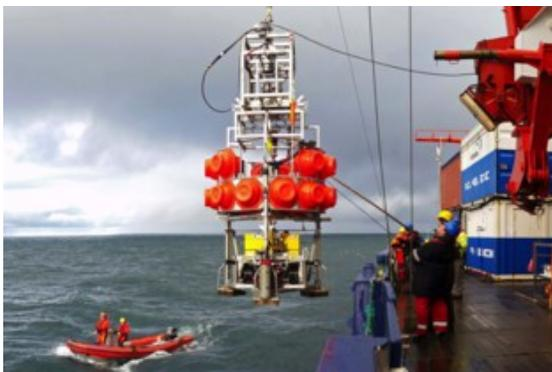
On the evening of September 4 we had a second test mission of the new robotic system MANSIO-VIATOR (Fig. 5). The system was developed within the HGF-Alliance ROBEX and consists out of a deep-sea crawler „VIATOR“ and a non-mobile lander „MANSIO“. This was the first time the system was deployed in a water depth of 1276 m
