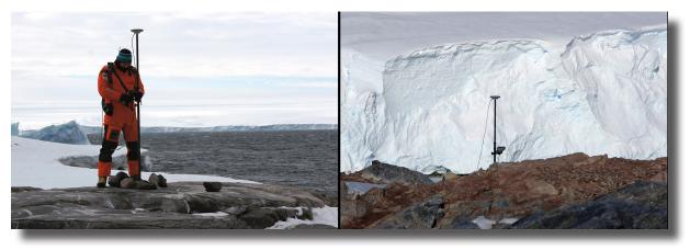
Fig. 9.3: GPS real-time kinematic (RTK). The antenna is mounted on a special rod of defined length that enables to marking the location to be measured. The receiver is carried in a special bag. Left: Suchland Islands (site SU01), right: Molar Islands (site FE01)
