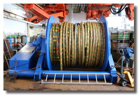
Fig. 6.2: Winch with 600 m long analogue streamer
