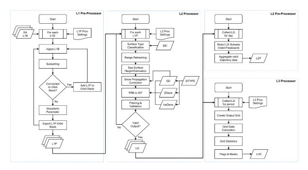
Figure 1: Workflow of the sea ice production system
