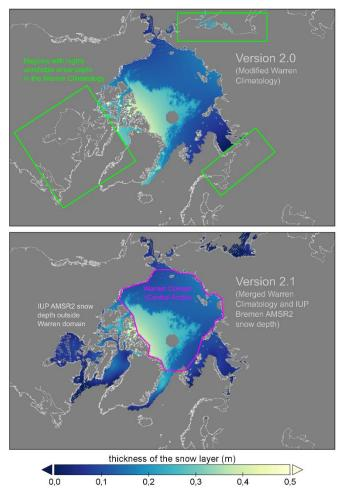
Figure 7: Comparison of W99 only (upper panel) used in v2.0 of the AWI CryoSat-2 sea ice product and merged W99 snow depth climatology (lower panel) modified by sea ice type introduced in v2.1. The merged Warren/AMSR2 snow depth climatology improves the snow depth information in areas outside the domain of the W99 climatology (central Arctic Basin)
