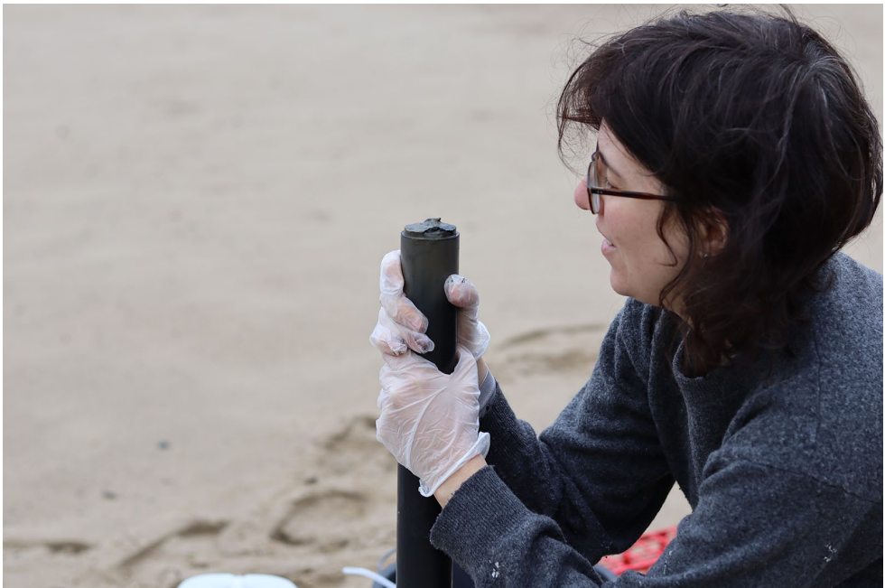
Figure 4. Anna pushing the corer slowly down the solid tube to expose the topmost layers of sediment. Photograph by Amelia Hine.
