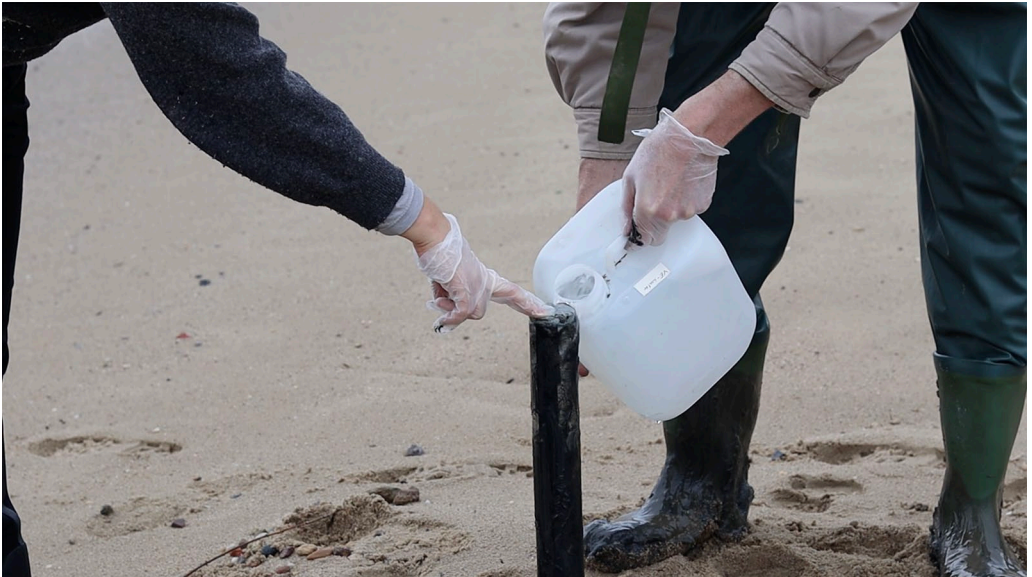
Figure 6. Thorsten and Anna using clean freshwater to try to wash the mud off the push corer exterior. Video still by Amelia Hine.
