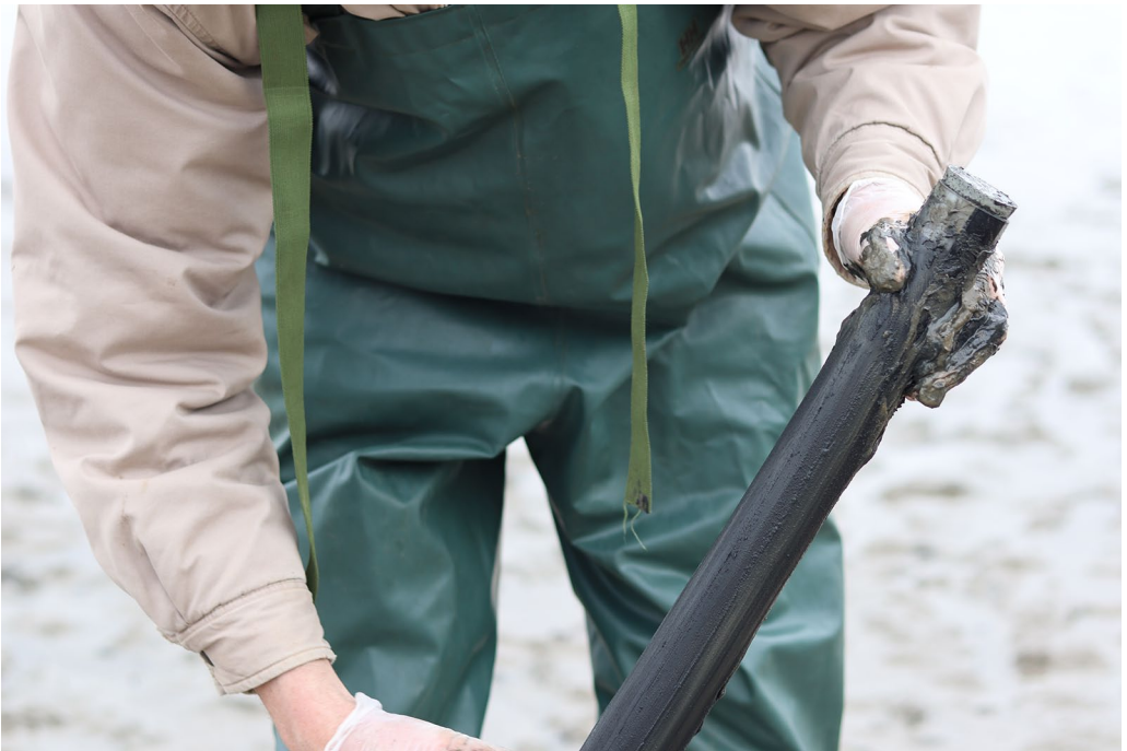
Figure 2. The rubber stopper sealing the top of the corer after extraction. Photograph by Amelia Hine.
