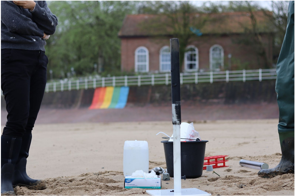
Figure 3. The corer filled with sediment atop the solid tube used to push the sediment out. Photograph by Amelia Hine.
