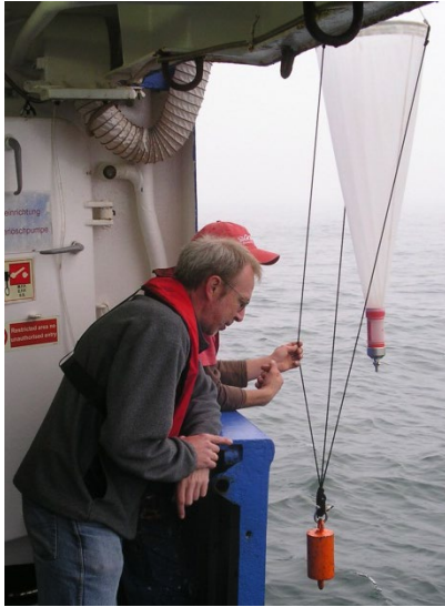
Plankton net pore size 20 \mu\text{m}
