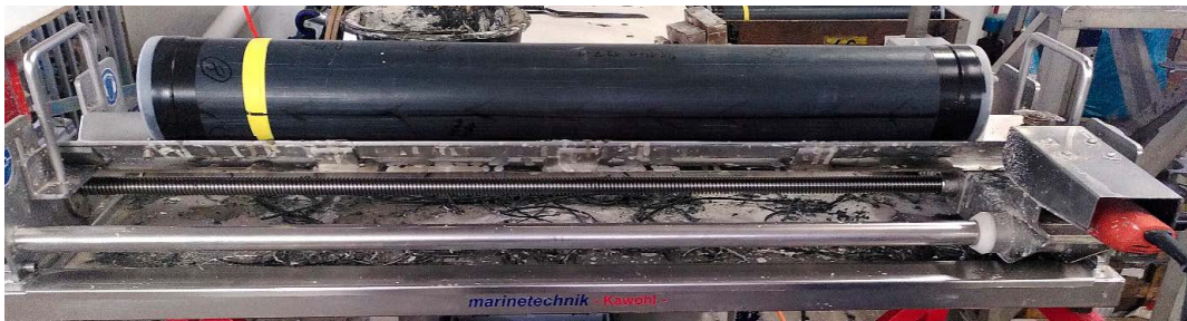
Fig. 5.14: Splitting of a core section in working and archive halves, using the Fa. Marinetechnik Kawohl vibration saw tool
