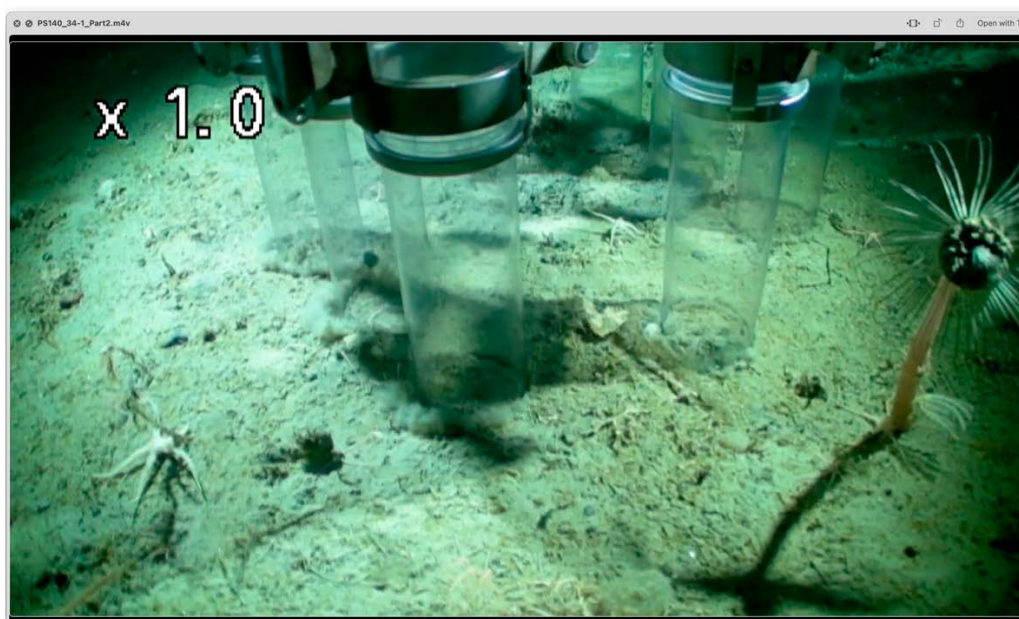
Fig. 5.7: TV-MUC deployment at station PS140_34-1, still from video at bottom penetration, note the relatively abundant benthic macrofauna on this site.
