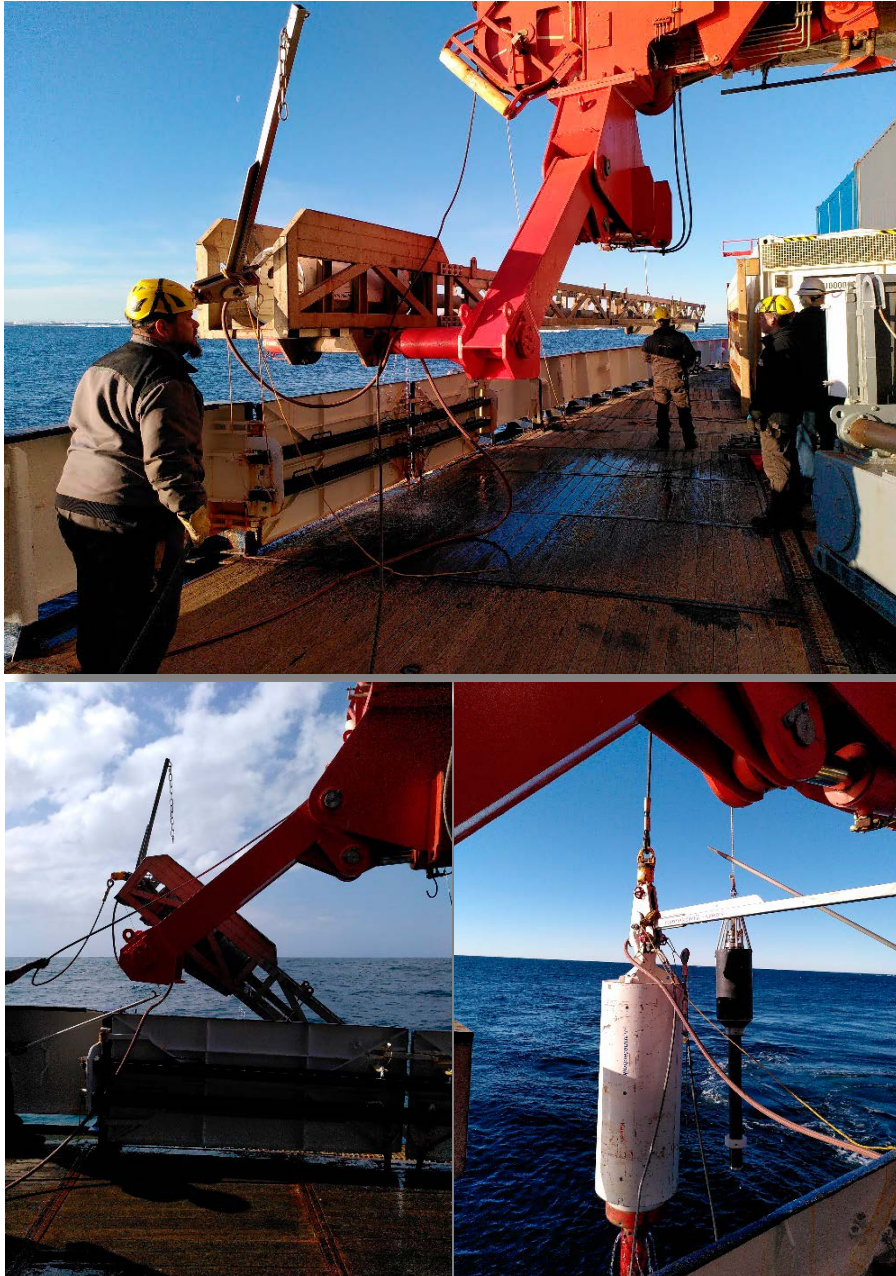
Fig. 5.9: Polarstern's core handling rack system to deploy long coring devices, here the piston corer
