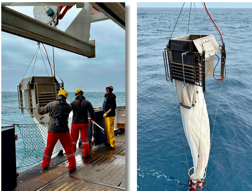
Fig. 5.1: Deployment and retrieval of Hydrobios Multi-Net during PS140
