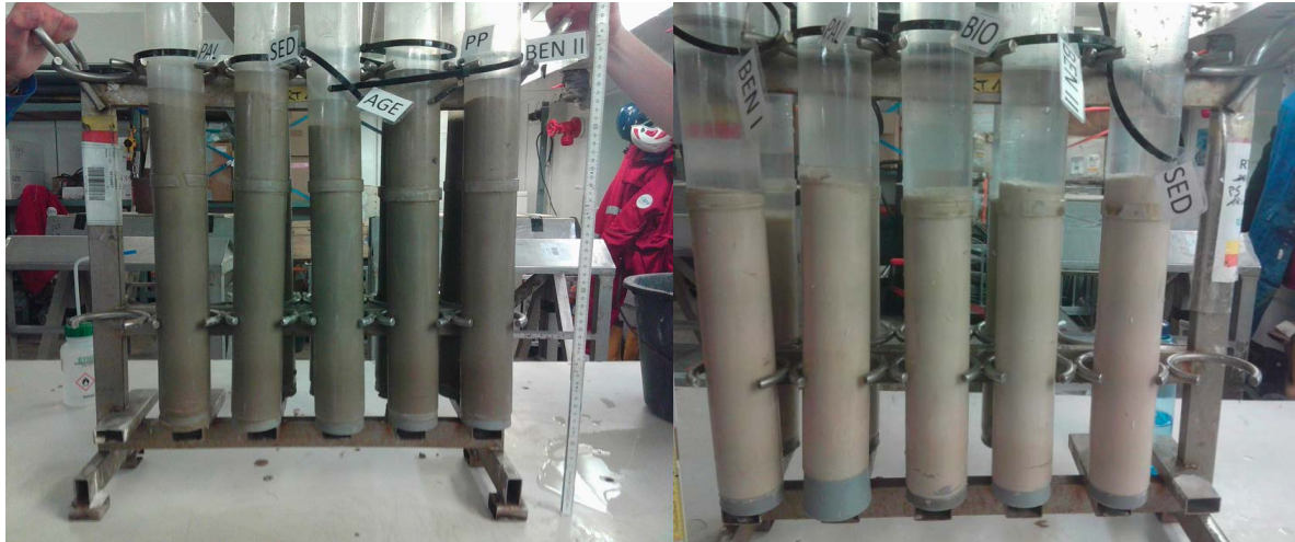
Fig. 5.5: Examples of photo-documented MUC tubes retrieved at station PS140_14-4 (left) and PS140131-2 (right). Note the evident optical differences in bio-siliceous-terrigenous vs. carbonate-dominated sedimentary facies
