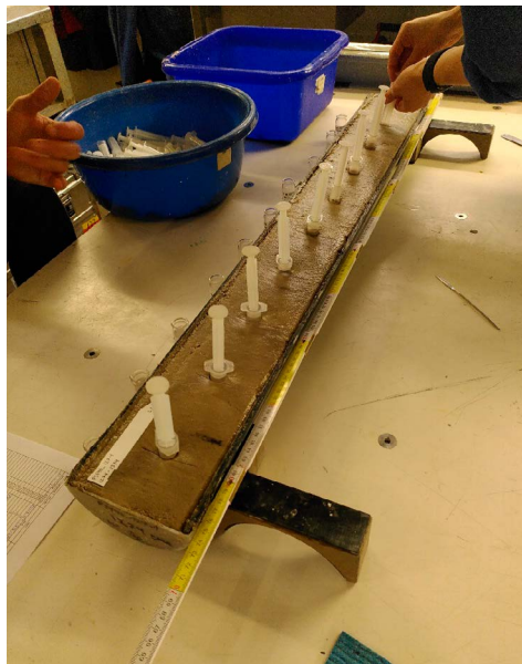
Fig. 5.15: Sampling of the working half in 10 cm distances with syringes of 10 mm diameter
