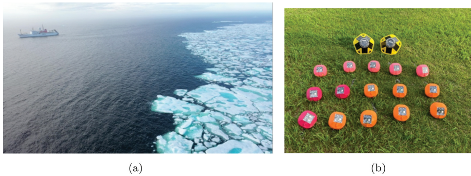
Figure 4. (b) Photograph taken by Tomotaka Katsuno showing the sea ice edge where wave buoys were deployed from R/V Mirai in MR22 cruise. (b) wave buoys prepared for the MR22 cruise. Although only two Spotter buoys are shown in the photo, three Spotter buoys were deployed.
